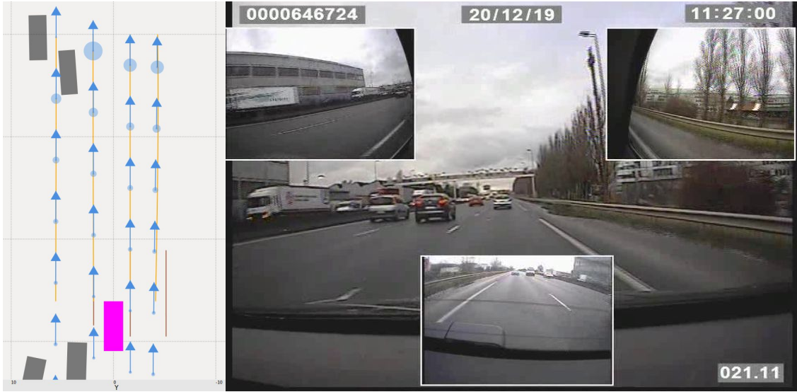
Figure 3.11: On the left, tracking results (blue) and measurements (orange for FrontCam, brown for AVM) are displayed in a bird-eye view. On the right, the context cameras.
