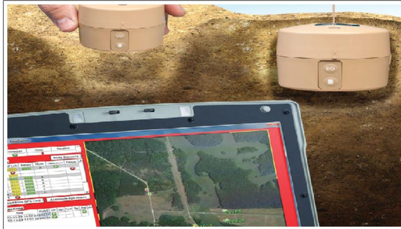
FIGURE 1.13 – The E-UGS Seismic Sensor Node.
