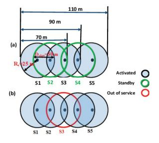
FIGURE 3.7 - (A): Scalar sensors deployment (03 activated sensors and 02 in standby mode) (B): If S3 fails, its area is monitored by S2 and S4.
