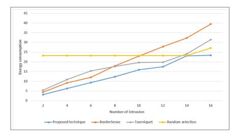
FIGURE 3.18 – Network energy consumption (in joule) vs the number of intrusions.
