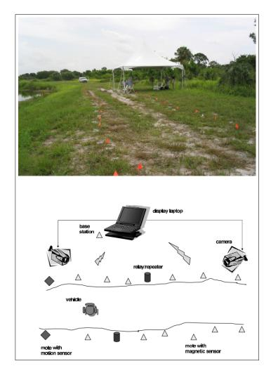
FIGURE 2.8 – Magnetic wireless sensor network for border surveillance.
