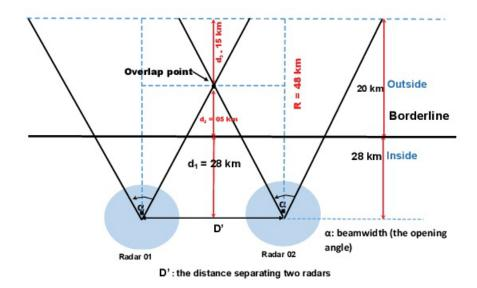
FIGURE 3.8 – Radars deployment : The overlapping area between two consecutive radars.
