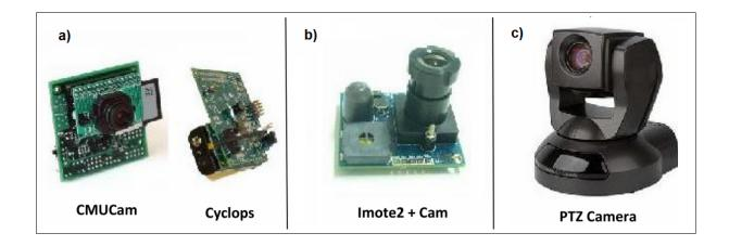
FIGURE 1.17 – a) : Low-resolution Camera; b) : Intermediate-resolution Camera; c) : High-resolution Camera.
