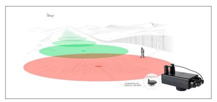
FIGURE 1.12 – The RS-U Seismic Sensors Node.
