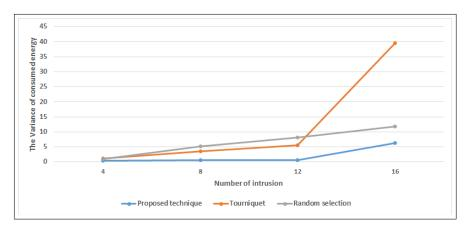
FIGURE 3.20 – Load balancing : The Variance of consumed energy by nodes.
