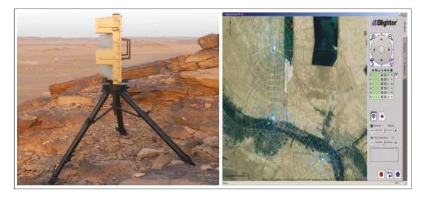
FIGURE 2.16 – Blighter scanning radar.
