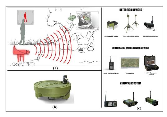
FIGURE 2.15 – (a) : Architecture deployment (an example), (b) :RS-N Directional Seismic Sensor, (c) The three main parts of the system.
