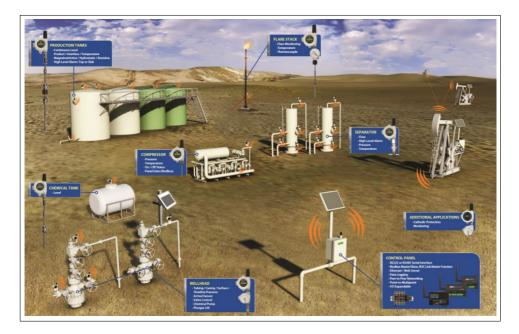
FIGURE 1.7 – WSNs Oil and gas applications.
