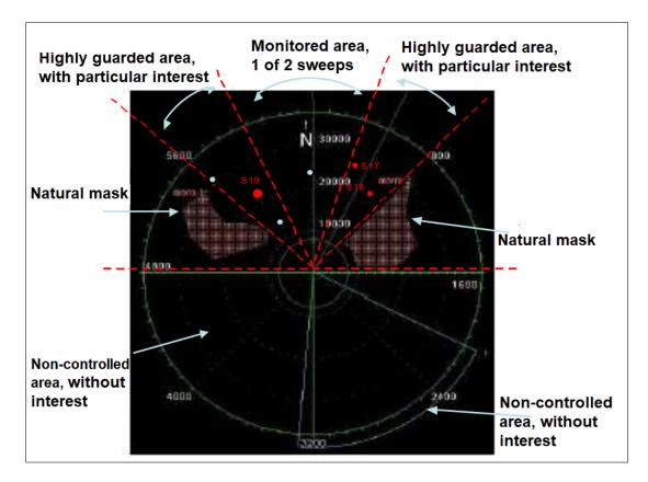
FIGURE 1.14 – Radar detection principle.
