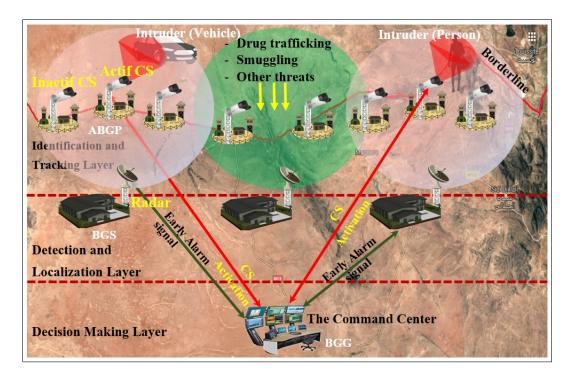
FIGURE 3.4 – Proposed network architecture of *Part02*.
