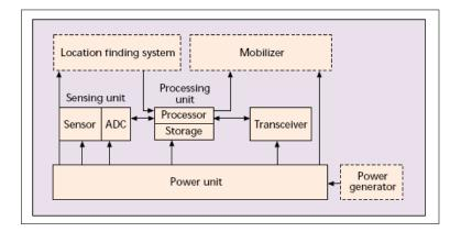
FIGURE 1.1 – Basic architecture of a sensor node.
