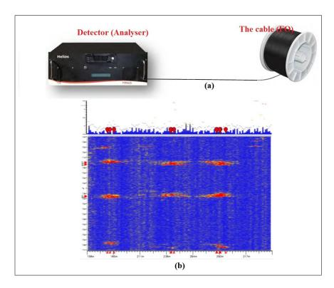
FIGURE 2.13 - (a): The two main parts of Helios , (b) :Screen shot of Helios system for two horses ran across the buried fiber optic cables.
