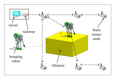
FIGURE 1.8 – WSN combined with jumping robots[4].
