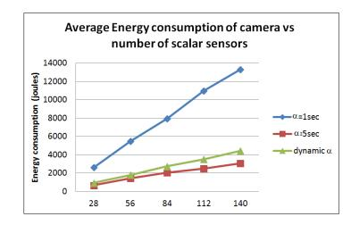
FIGURE 4.3 – Average energy consumption of a camera function of k.
