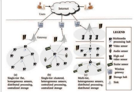
FIGURE 1.10 – Basic architecture of WMSN.
