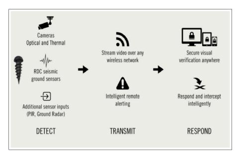
FIGURE 2.10 – Architecture of the EdgeVis Shield platform.
