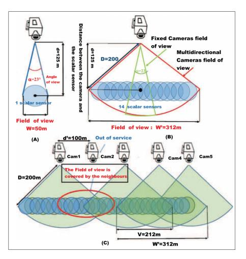
FIGURE 3.6 - (A): Field of view of a fixed camera (B): Field of view of a multidirectional camera (C): Overlapping area between two consecutive cameras
