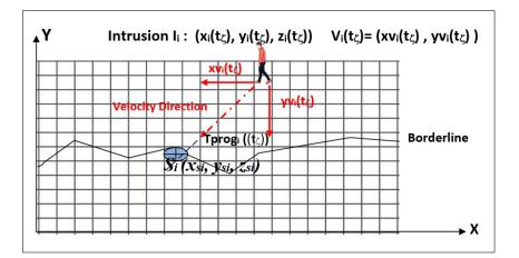
FIGURE 3.15 – Illustration of the calculation principle of the intruder progression parameter in the area of interest.
