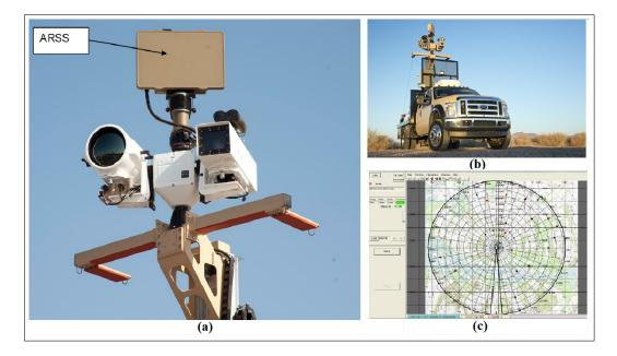
FIGURE 2.18 - (a): ARSS radar integrated with surveillance cameras, (b): ARSS integrated on Telephonics'RaVEN-msc!, (c): ARSS Interface showing the 360° coverage.
