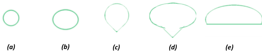
Fig. 1.21 Representative shapes of the single bubble in Newtonian fluid (a) spherical, (b) ellipsoidal, (c) teardrop shape, (d) flat teardrop shape with a pointed ellipsoid, (e) spherical cap.
