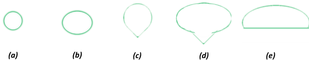
Fig. 1.21 Representative shapes of the single bubble in Newtonian fluid (a) spherical, (b) ellipsoidal, (c) teardrop shape, (d) flat teardrop shape with a pointed ellipsoid, (e) spherical cap.
