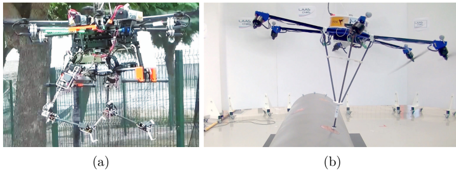
Figure 1.4: Second generation of aerial manipulators: (a) An aerial dual-arm manipulator with compliant joints [Ollero 2018]; (b) A fully actuated platform interacting with the environment [Ryll 2019]
