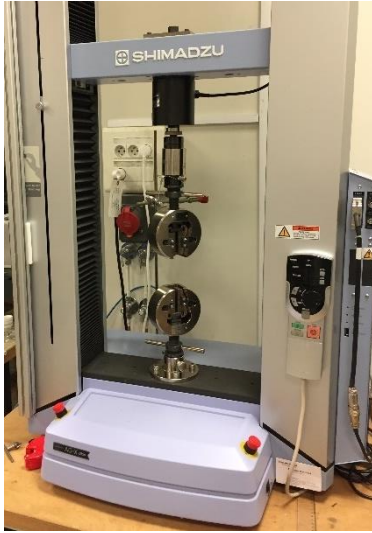
Figure II - 17: Mechanical traction tests on injected composite material dog bones. Left: Tensile test equipment. Right: Load curve of PP – 2.5 vol% sample with experimentally measured mechanical properties.
