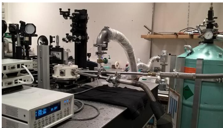
Fig2.2 Cold finger cryostat fixed onto movable stages. The chamber is connected by two parallel circuits to a pumping blocs seen in the background and to a He vessel, on the right. The Lakeshore temperature controller can be seen at the bottom left of the picture.
