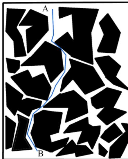
Figure 9 Scheme of tortuosity in a porous media. the blue line describes a viable path for a chemical species from point A to B.
