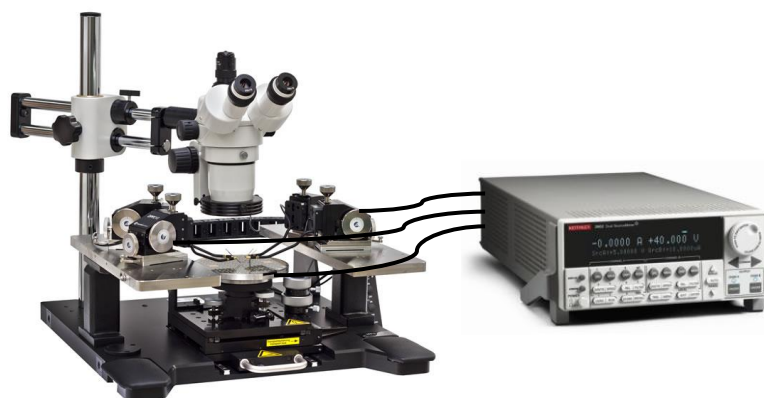
Figure 5.8. Schematic representation of the Current-Voltage (I-V) characterization set-up which consists of a Cascade Microtech M150 probe station connected with a dual channel Keithley 2636A source-meter and its associated software.
