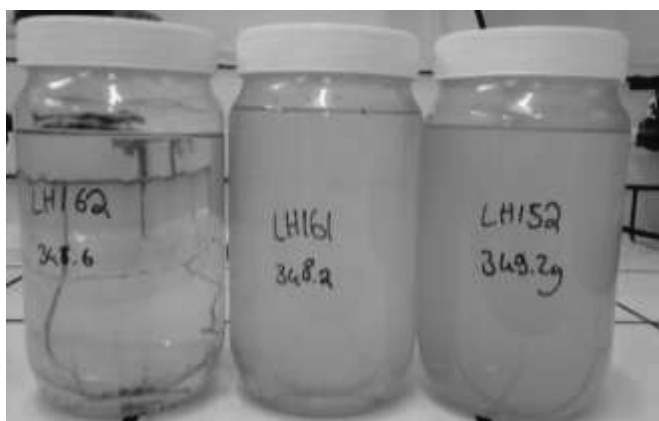
Figure 62: Example of clear and hazy resins due to reaction procedures
