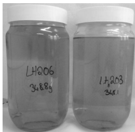
Figure 25: Highly coloured isosorbide resins synthesised from isosorbide stored for several months
