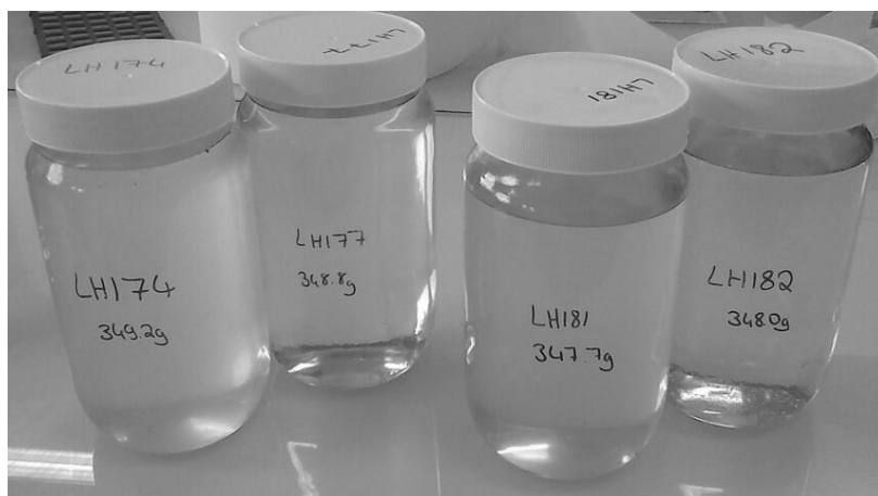
Figure 22: Colourless and transparent resins based on phthalic anhydride (LH174 – LH182)
