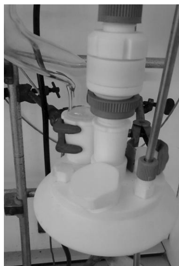
Figure 28: Teflon reactor top
