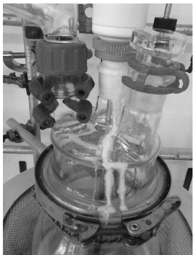
Figure 27: Leak in reactor with new joint
