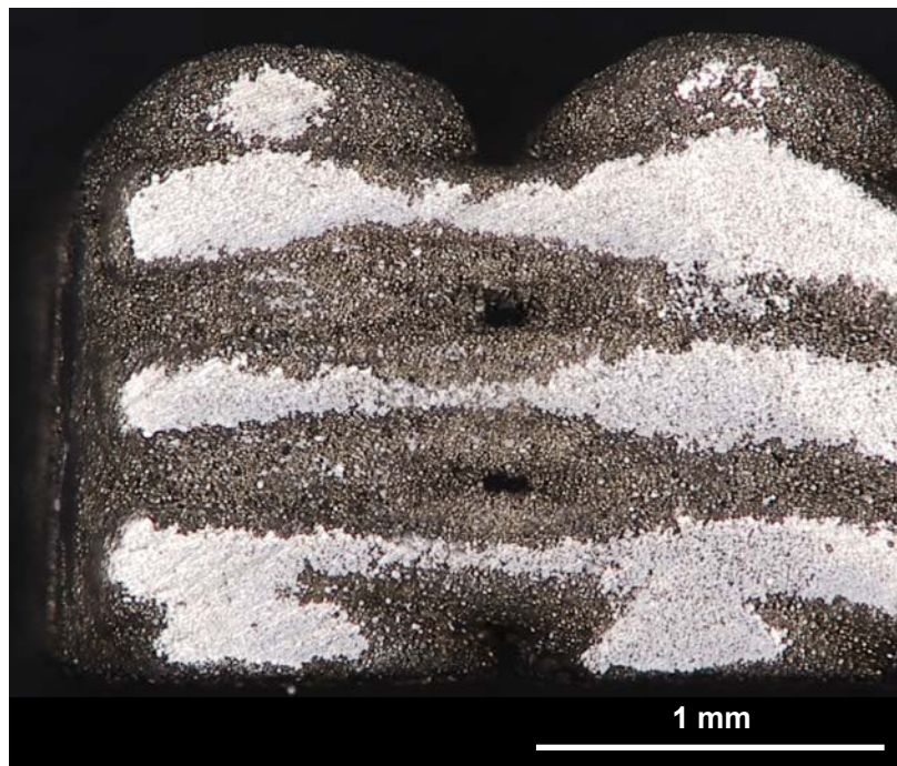
Figure 4.17: Photo taken with a binocular magnifying glass after lightly polishing one side of the SPS-sintered scaffold. White areas correspond to the areas in cross-section, which were in the polishing plane.
