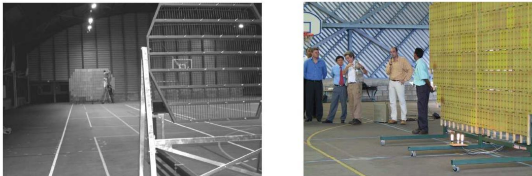
FIGURE 1.3: Demonstration of Grand Bassin: Overview (right) and array of 2376 rectennas (left) [5].
