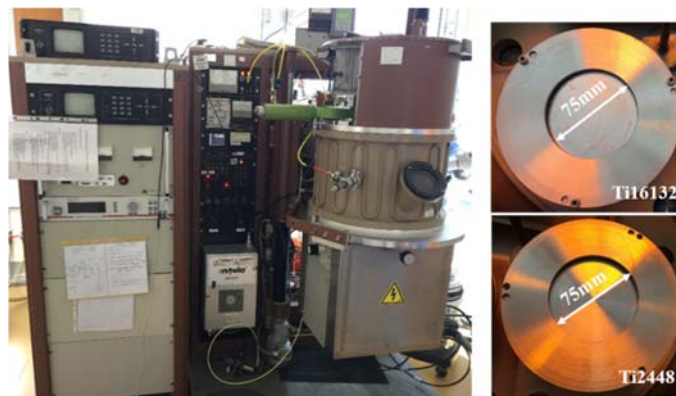
Fig. II-9 RF magnetron sputtering machine and the alloy targets for Ti16132 and Ti2448 films.
