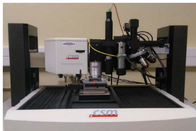
Fig. II-20 Anton Paar TriTec mechanical platform for surface and mechanical characterizations.
