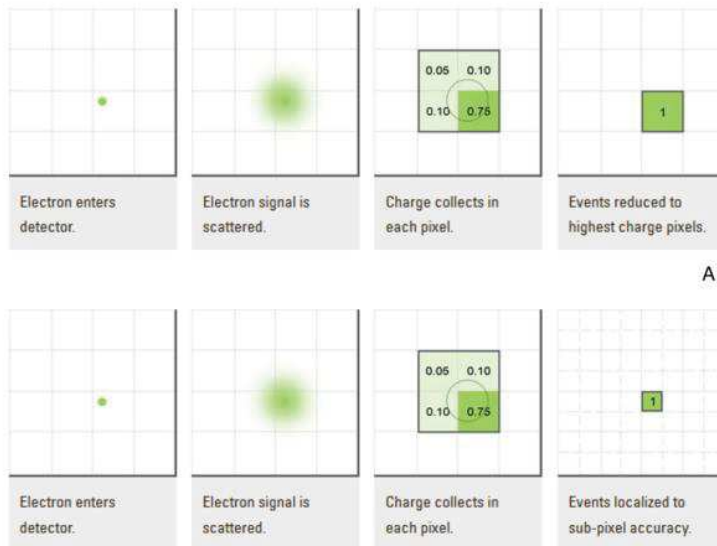
Figure 3-12 Detectors imaging modes
