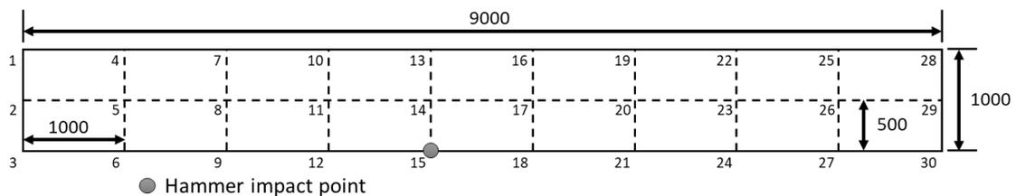
Figure 3.3. Accelerometer layout with the hammer impact location
