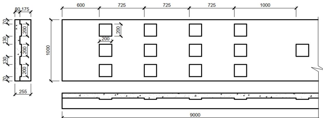
Figure 4.2. Connector layout of the tested CCC specimen [155]
