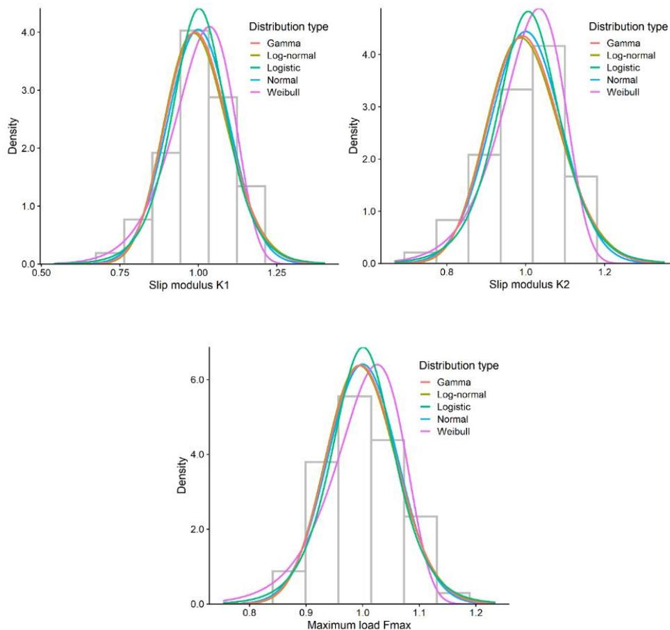
Figure A2.1. Dimensionless distribution of slip modulus K1, K2, and maximum load Fmax
