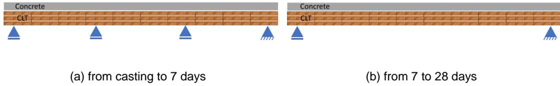
Figure 3.2. Schematic plan of the supports at the early and later state of the beam
