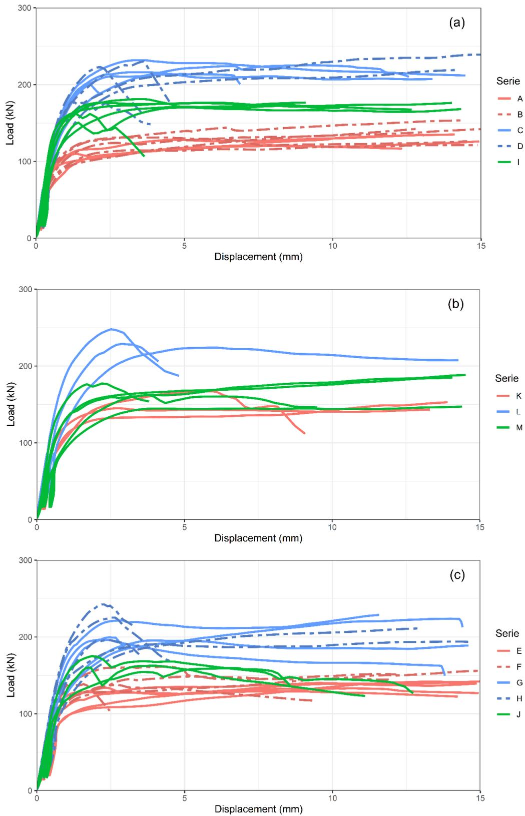
Figure 2.5. Load-displacement curves of specimens that have (a) 400 mm, (b) 350 mm, (c) 300 mm heel length, curves in red indicate 20 mm notch depth specimens, 25 mm in green, and 35 mm in blue.
