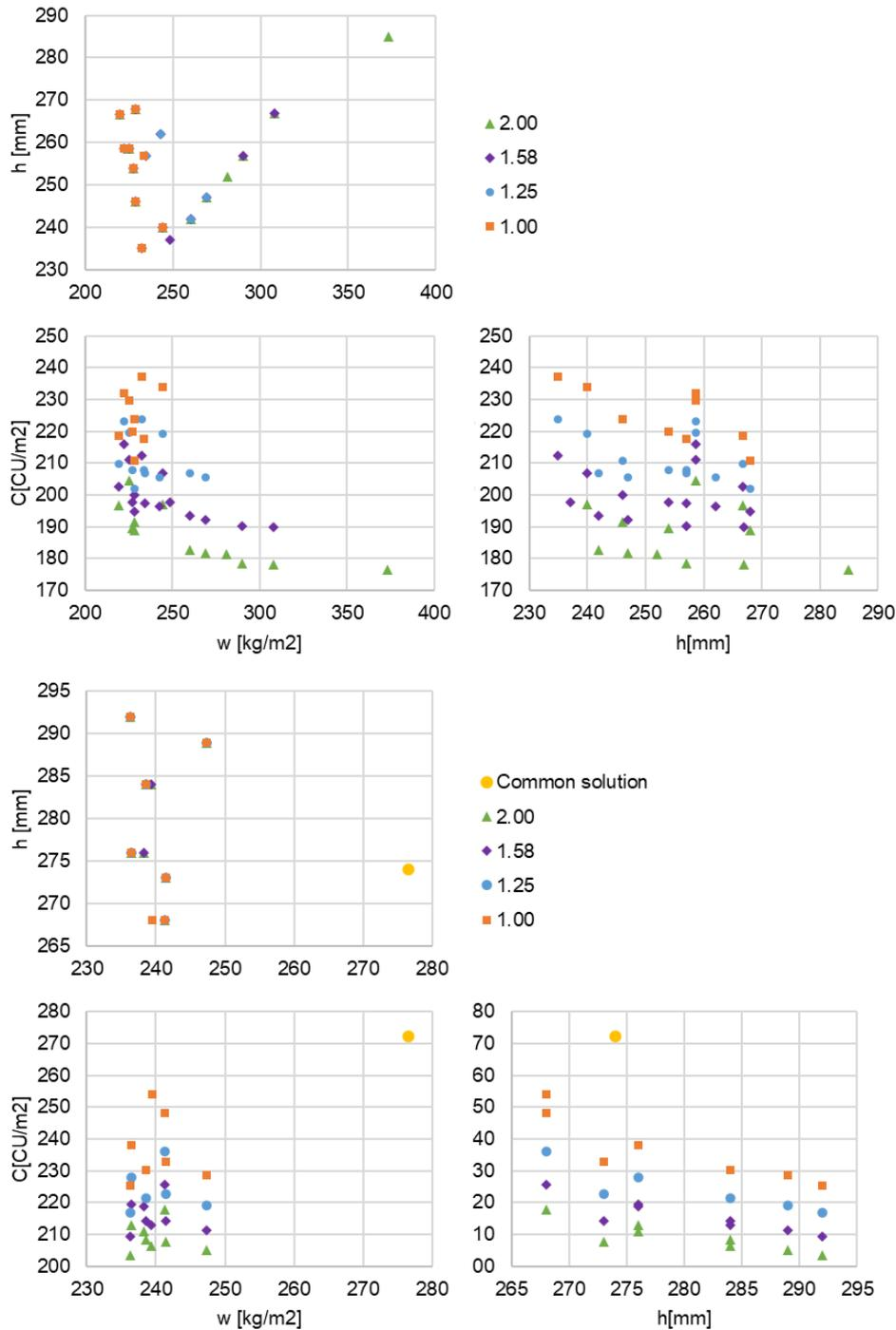
Figure 4.8. Pareto fronts of different ratio Timber/Concrete for 8 m (top) and 9 m (bottom) floor span
