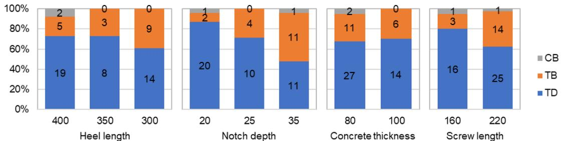
Figure 2.14. Number of specimens with different failure types.
