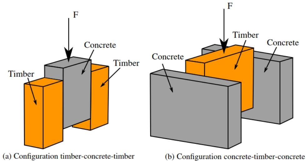
Figure 1.15. Configuration symmetric for shear connector tests, adapted by C. Auclair [43]
