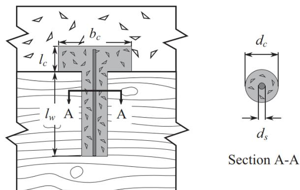
Figure 1.12. Notched connector geometry, by C. Auclair *et al.* [63]
