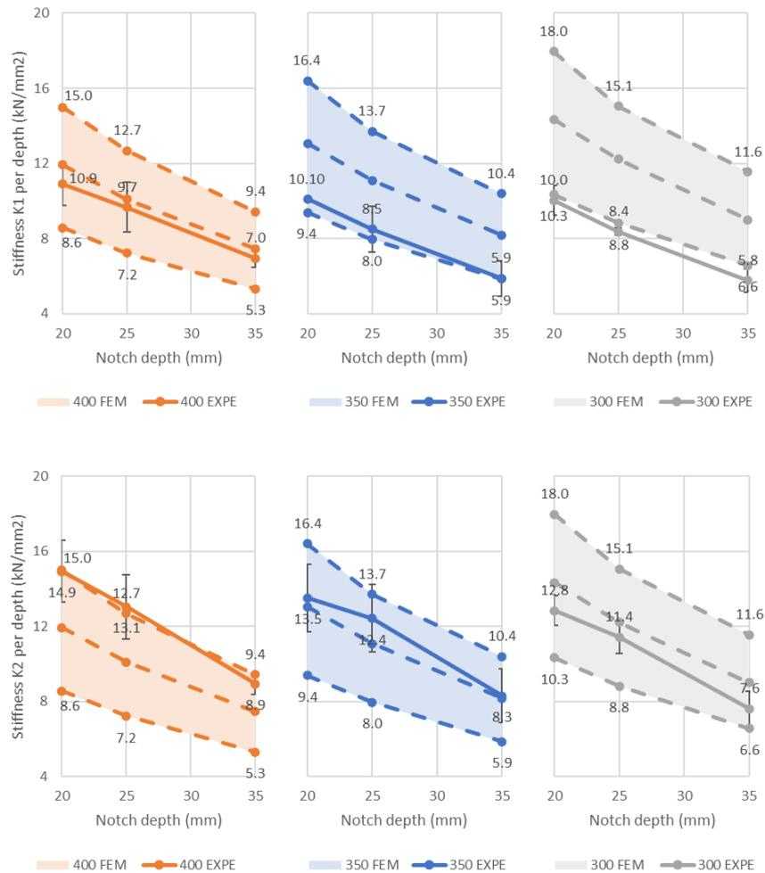
Figure 2.16. FEM envelop of stiffness K1 and K2 per depth of multiple heel length.
