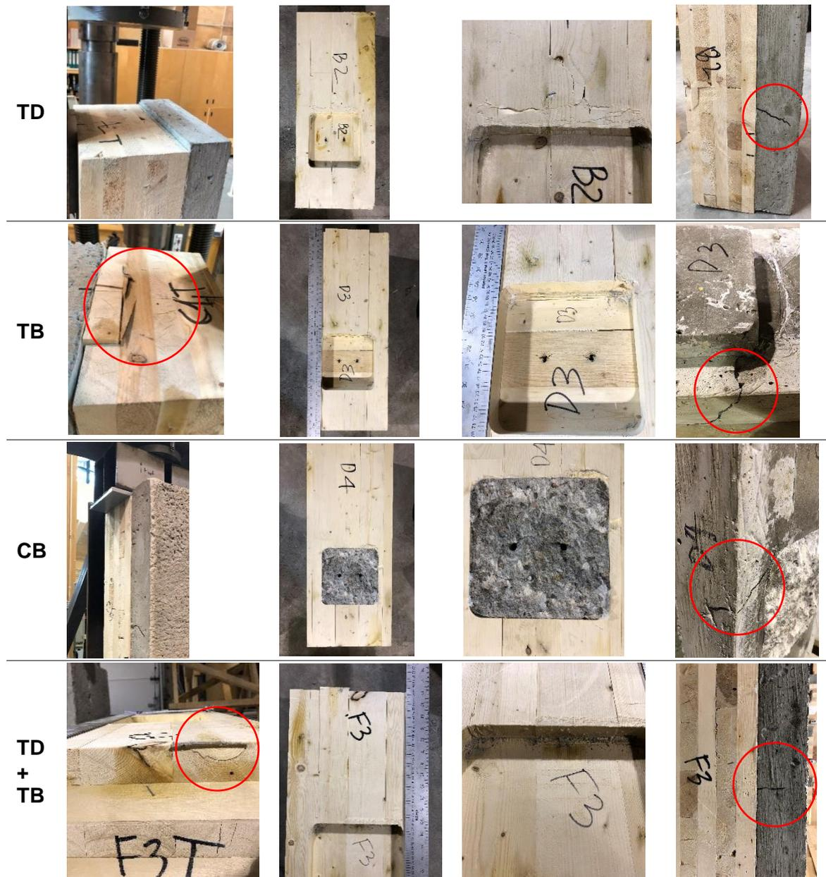
Figure 2.13. Typical different failure types.
