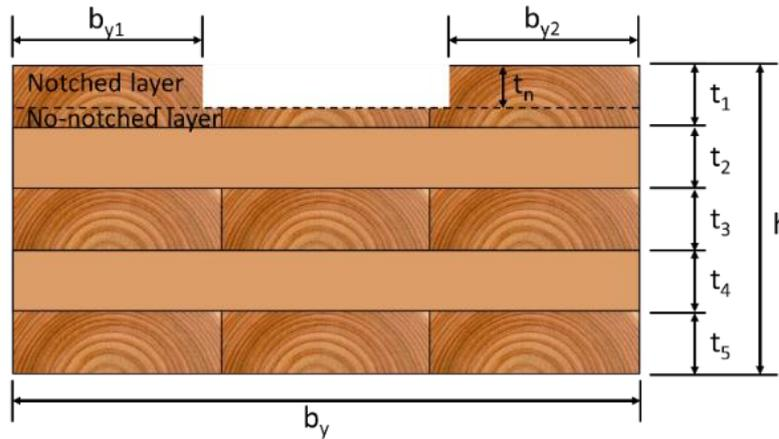
Figure 3.4. Cross-section of notched beams
