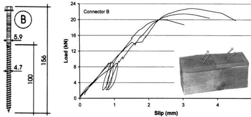
Figure 1.4. Load-slip curves of SFS screws (A) and regular screws (B) by Steinberg *et al.* [49]
