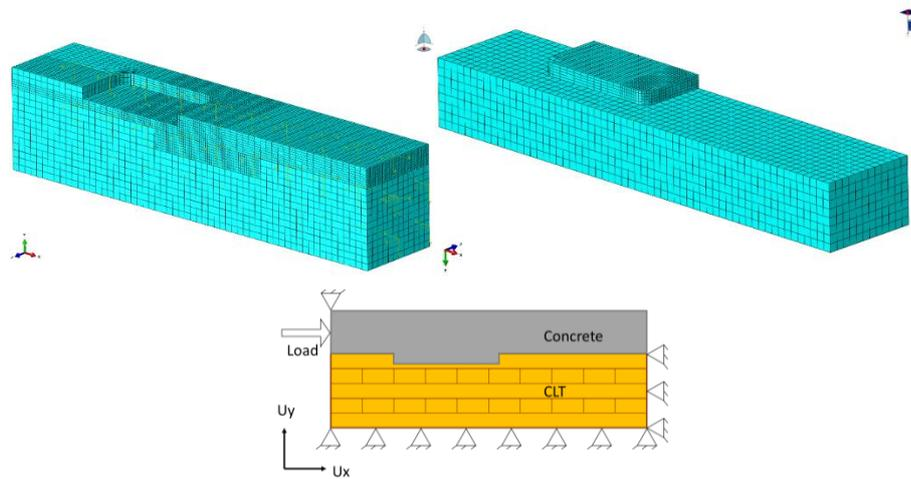
Figure 2.15. Mesh definition of timber and concrete part and boundary conditions.
