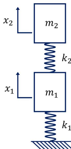
Figure 1.13. A simple two-degree-of-freedom system model.
