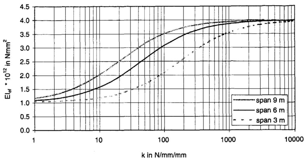
Figure 1.2. Relationship between the effective bending stiffness of the composite beam and the slip modulus on a logarithmic scale, per Van der Linden [24].
