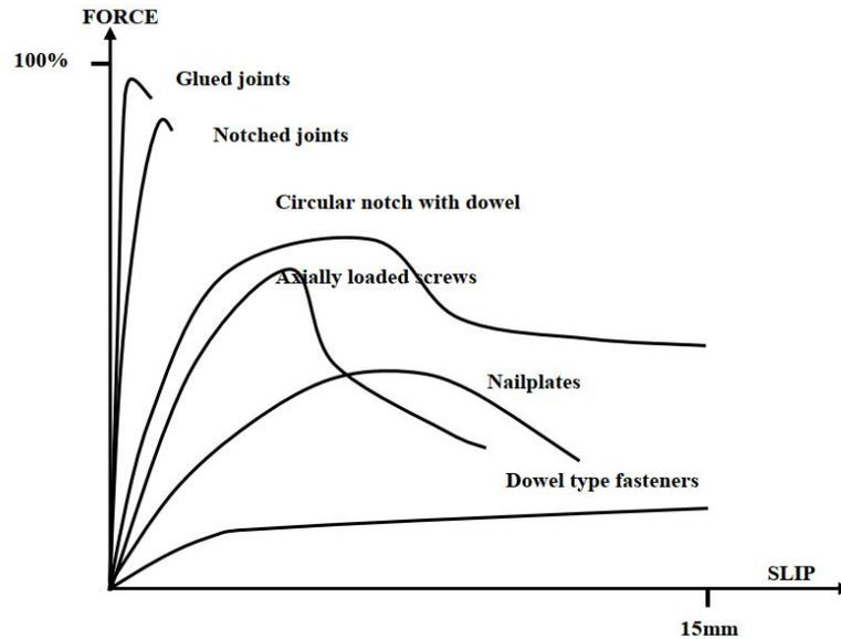
Figure 1.3. Comparison of different types of typical TCC connectors by Dias [25].
