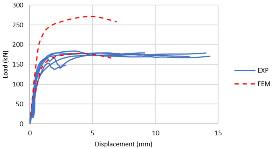
Figure 2.18. Load-displacement curves comparison between experimental and FEM of series I.
