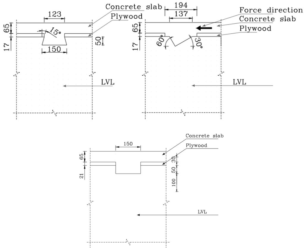
Figure 1.10. Three geometry form of notch connectors, by Yeoh [60]
