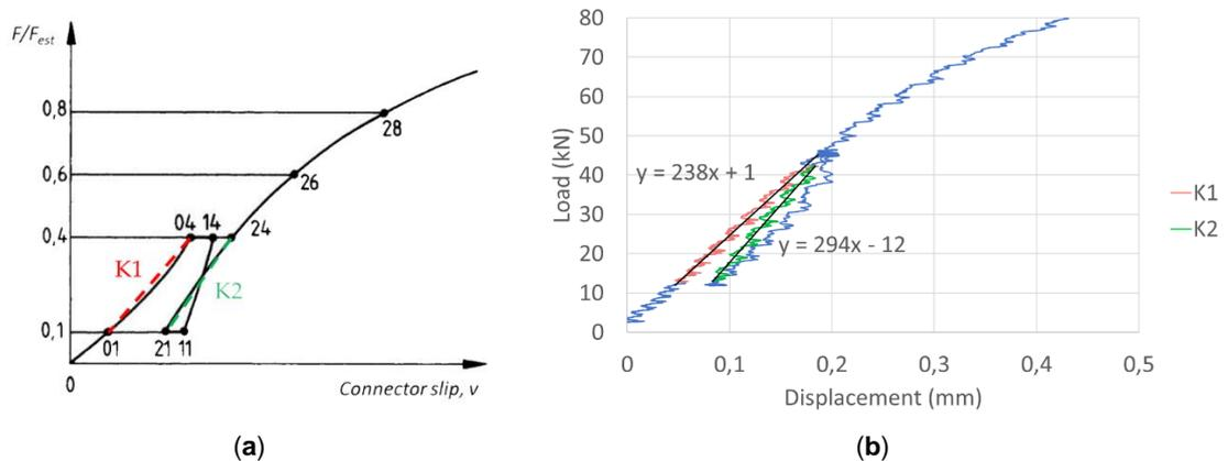
Figure 2.4. Theoretical loading procedure from EN 26891 [95] (a) and stiffness  $K_1$  (red) and  $K_2$  (green) determination of specimen A2 (blue) on raw data representation (b).
