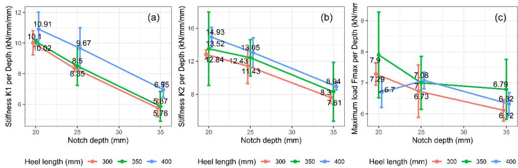
Figure 2.8. Stiffness K1 (a), K2 (b), and maximum load Fmax (c) per notch depth of different heel lengths.
