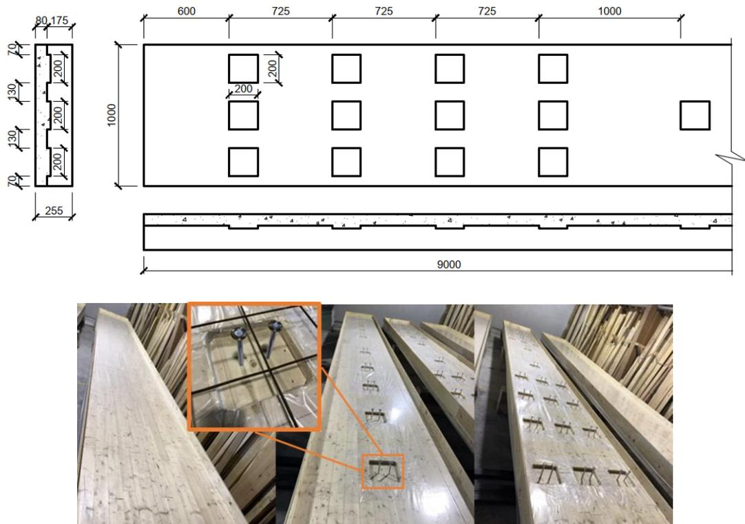
Figure 3.1. Connector layout of Beam 3 and actual image of the beams before concrete casting
