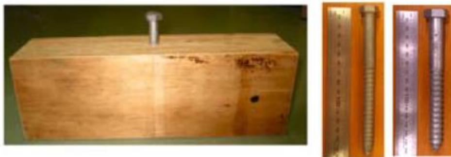
Figure 1.6. Lag screws connectors, by Deam *et al.* [58]
