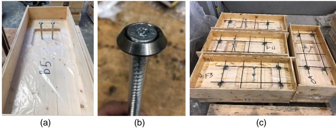
Figure 2.1. Specimen with preinstalled polyethylene film (a), vertical attachment part with a threaded screw, counter-sunk washer and plastic sleeve installed (b), reinforcing steel mat of the specimens (c).
