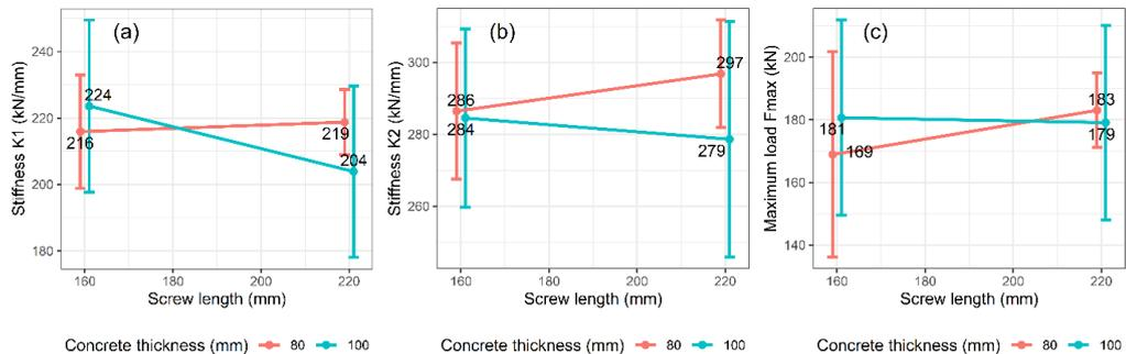
Figure 2.9. Stiffness K1 (a), K2 (b), and maximum load Fmax (c) in terms of screw length and concrete thickness
