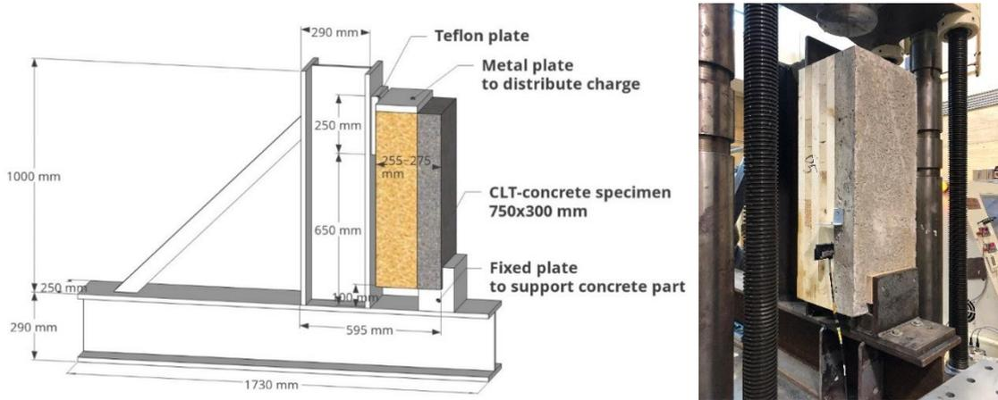
Figure 2.3. Adaptor for the asymmetrical CLT-concrete specimen (left). Actual image of adaptor (right).
