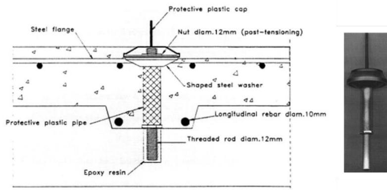
Figure 1.11. Notch with dowel connectors and image of Hilti dowel, by Gutkowski *et al.* [62]
