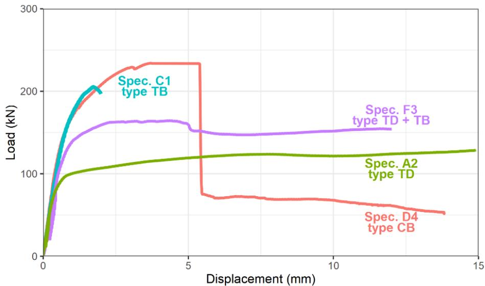
Figure 2.12. Load-slip curves of different failure types.
