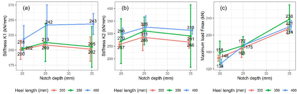
Figure 2.7. Stiffness K1 (a), K2 (b), and maximum load Fmax (c) of different heel lengths.
