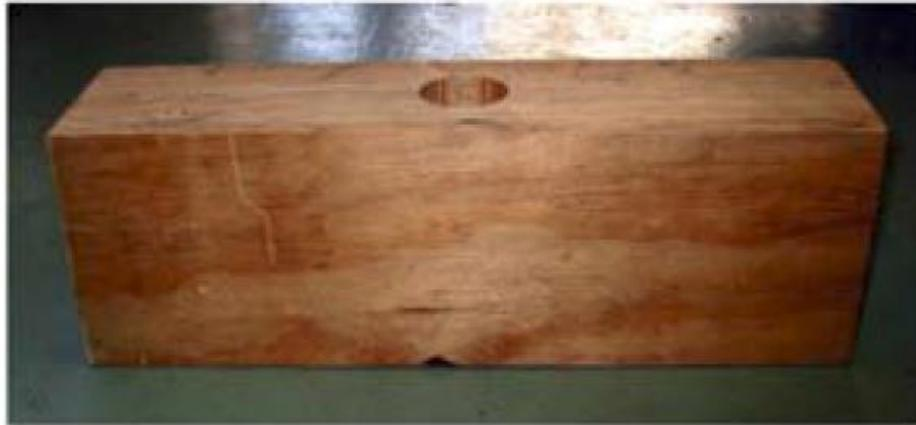
Figure 1.9. Round notch (or plug) connector, by Deam *et al.* [58]
