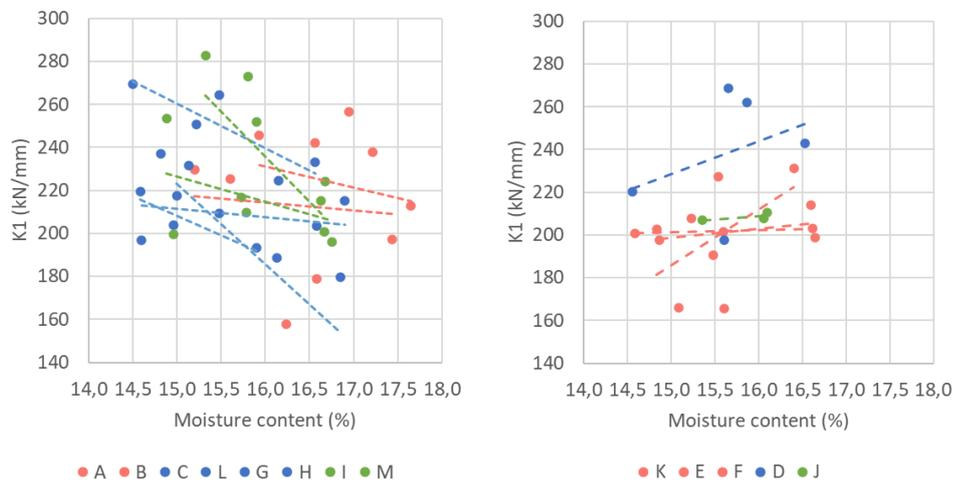
Figure 2.11. Correlation between stiffness K1 and moisture content of timber of different series. 20 mm notch depth specimens are represented by the red points, 25 mm in green, and 35 mm in blue.
