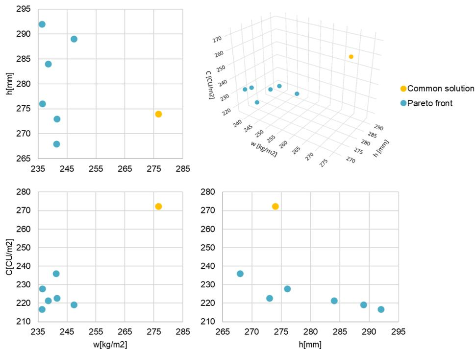
Figure 4.5. Pareto front of CLT-concrete solution for 9 m floor span
