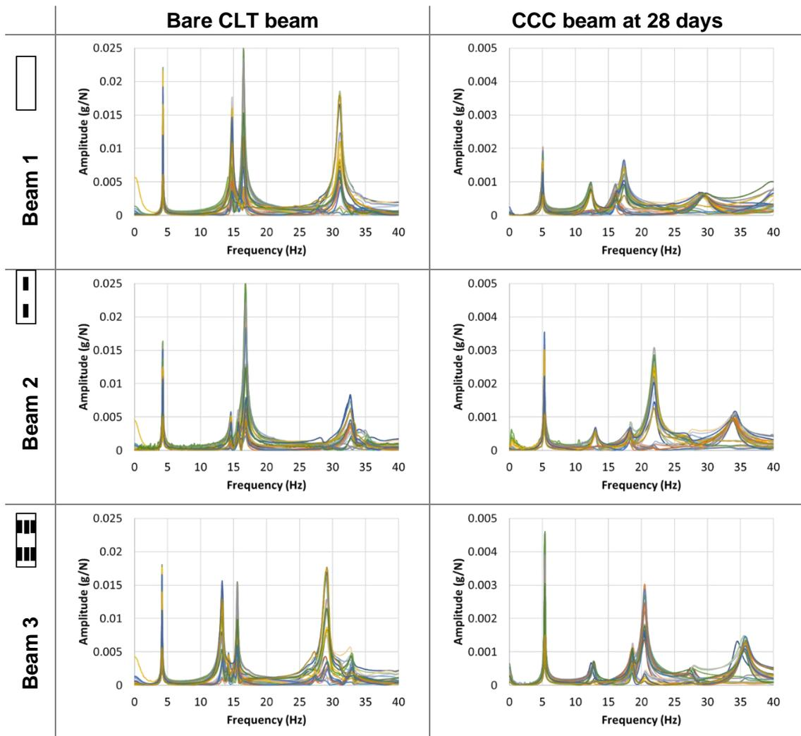
Figure 3.7. Frequency response functions (FRF) from 24 measurement points of bare CLT beams and CCC beams 28 days after concrete casting
