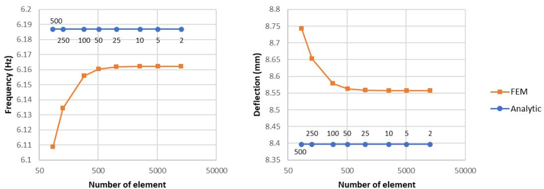
Figure 3.6. Mesh sensitivity, data labels represent the corresponding element size
