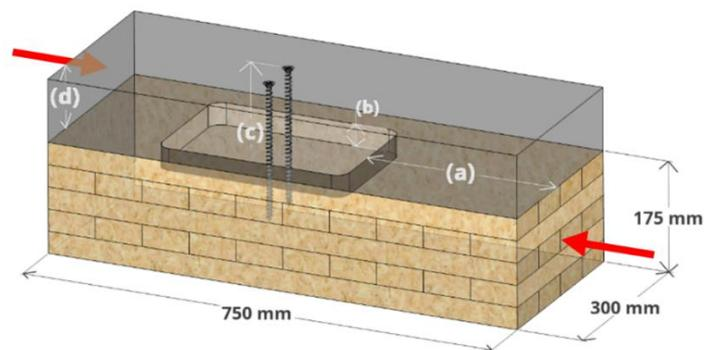
Figure 2.2. Diagram of a typical specimen, with indicated (a) heel length, (b) notch depth, (c) screw length, (d) concrete thickness.
