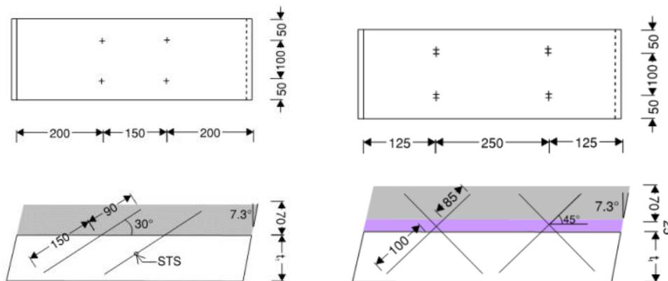
Figure 1.5. Specimens with STS at  $30^\circ$  and pairs of STS at  $45^\circ$  with insulation layer, by Gerber [59].
