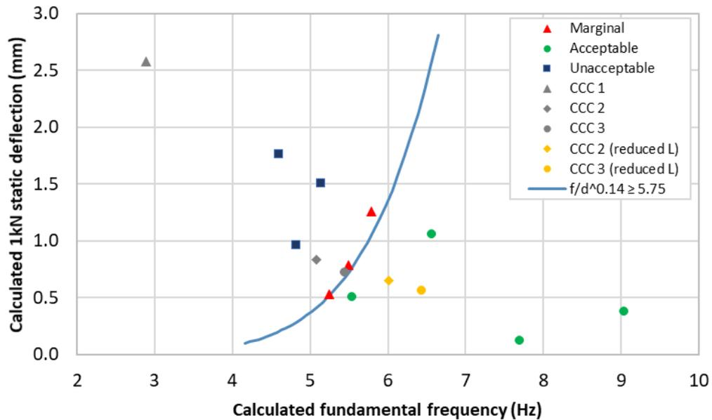
Figure 3.8. Proposed design criterion with subjective evaluations of CCC floors [127] and calculated results of this study
