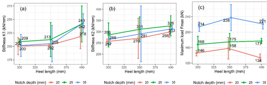
Figure 2.6. Stiffness K1 (a), K2 (b), and maximum load Fmax (c) of different notch depths.
