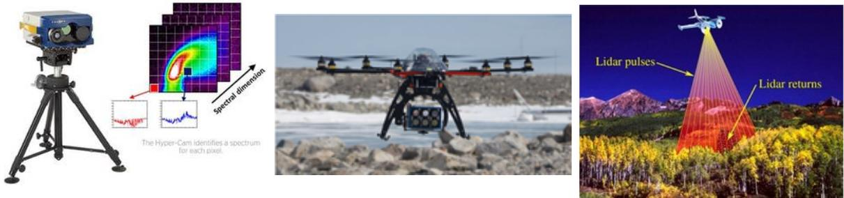
Figure 2: Optical instruments, from left to right: Hyperspectral Camera, multispectral camera and LIDAR.
