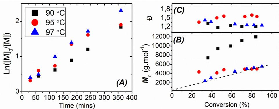
**Figure 5.1.** Polymerization of THGMA ( $[M]_0/[Disp\text{olreg } 007]_0 = 25$ ) in toluene,  $[M]_0 = 1.95 \text{ mol.L}^{-1}$  at 90 (Squares), 95 (Circles) and 97 °C (Up triangles). (A) Evolution of  $\text{Ln}[M]_0/[M]$  as a function of time. (B) Evolution of the measured molar masses as a function of monomer conversion. (C) Evolution of the dispersity values as a function of monomer conversion.
