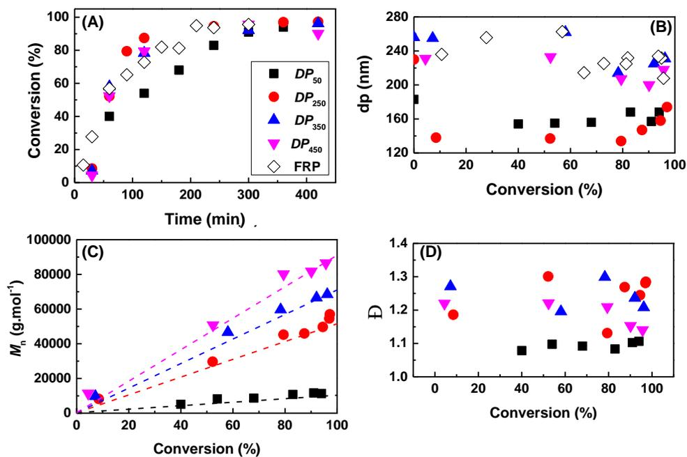
**Figure 4.3.** The kinetic plot of the poly(THGA) by RAFT miniemulsion polymerization at 70°C for 7 h with AIBN as an initiator at different targeted  $DP_n$ s;  $DP_{50}$  (Squares),  $DP_{250}$  (Circles),  $DP_{350}$  (Up triangles), and  $DP_{450}$  (Down triangles). (A) Conversion plot as a function of time. (B) Evolution of the particle size as a function of conversion. (C) Evolution of the molar mass as a function of conversion. (D) Dispersity values as a function of conversion.
