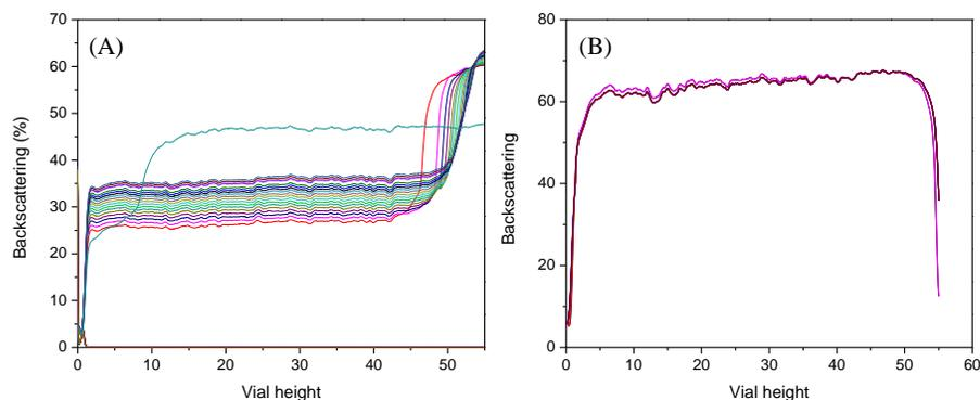
**Figure 4.1.** Stability of the THGA dispersion at 60 °C. The scans were conducted every 30 min for 5 h with 20 wt% solids content. (A) entry 1; 2 wt.% surfactant and 4 wt.% co-stabilizer. (B) entry 2; 3 wt.% surfactant and 5 wt.% co-stabilizer based on terpene acrylate.
