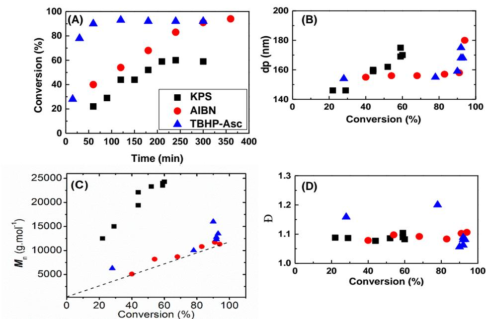
**Figure 4.2.** Kinetic of the RAFT miniemulsion polymerization of poly(THGA) with different initiators at 70°C,  $DP_n = 50$ ,  $[CTA]_0/[I_2]_0 = 10$ . (Squares) KPS; (Circles) AIBN and (Up triangles) TBHP/Asc. (A) Conversion plot as a function of time. (B) Evolution of the particle size as a function of time. (C) Evolution of the measured molar masses as a function of monomer conversion. (D) Evolution of dispersity values as a function of monomer conversion.
