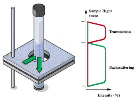
**Figure I.1** Representation of the Turbiscan Lab<sup>expert</sup> detection principle.
