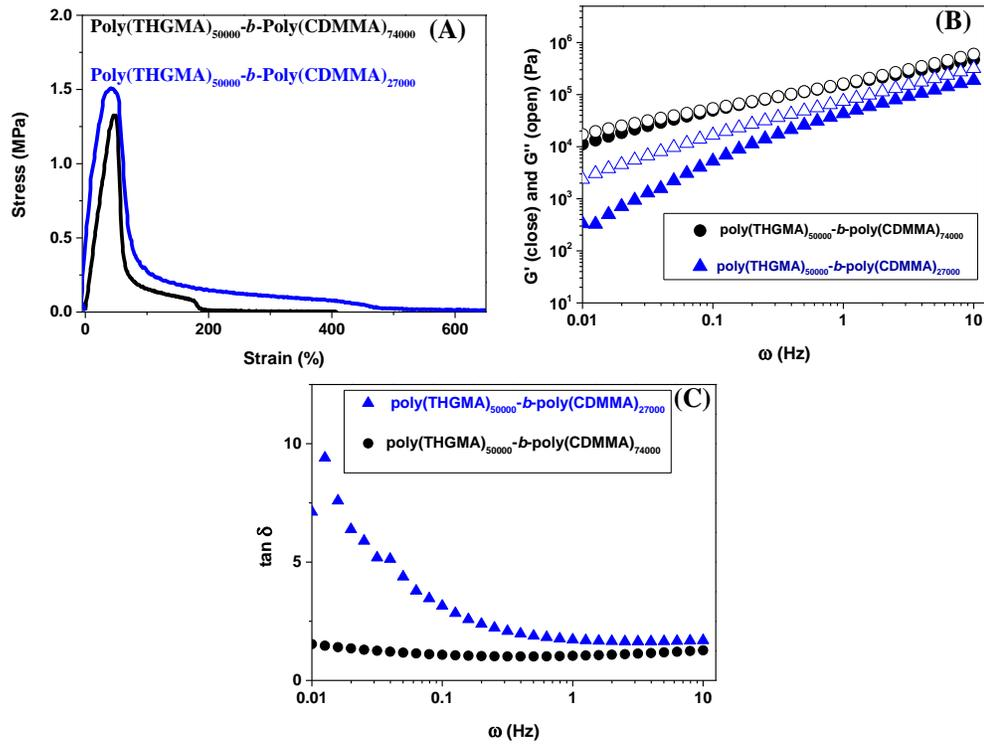
**Figure 5.10.** Evolution of adhesive properties for poly(THGMA)-*b*-poly(CDMMA) soft/hard diblock copolymer. (A) Stress-strain curve of the probe-tack test. (B)  $G'$  and  $G''$  as a function of frequency at room temperature. (C)  $\tan \delta$  as a function of frequency at room temperature.
