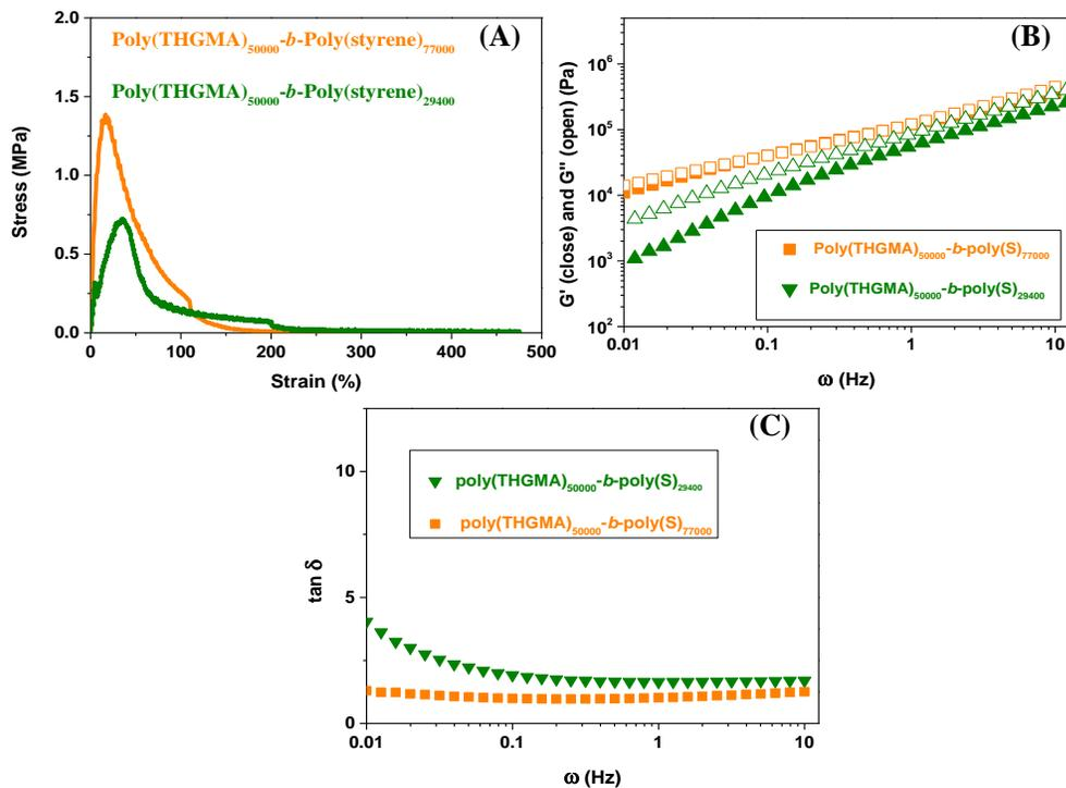
**Figure 5.11.** Evolution of adhesive properties for poly(THGMA)-*b*-poly(S) soft/hard diblock copolymer. (A) Stress-strain curve of the probe-tack test. (B)  $G'$  and  $G''$  as a function of frequency at room temperature. (C)  $\tan \delta$  as a function of frequency at room temperature.
