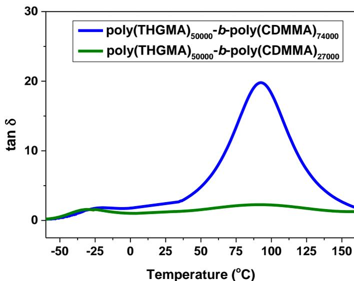
**Figure 5.8.**  $\tan \delta$  as a function of the temperature of the poly(THGMA)-*b*-poly(CDMMA) soft/hard diblock copolymer. The rheology of the block copolymers was performed using parallel plate geometry with constant strain on a rotational rheometer (TA ARES). Mechanical spectroscopy experiment was performed at frequency 0.1 rad/s over the temperature from 160 to -60 °C.
