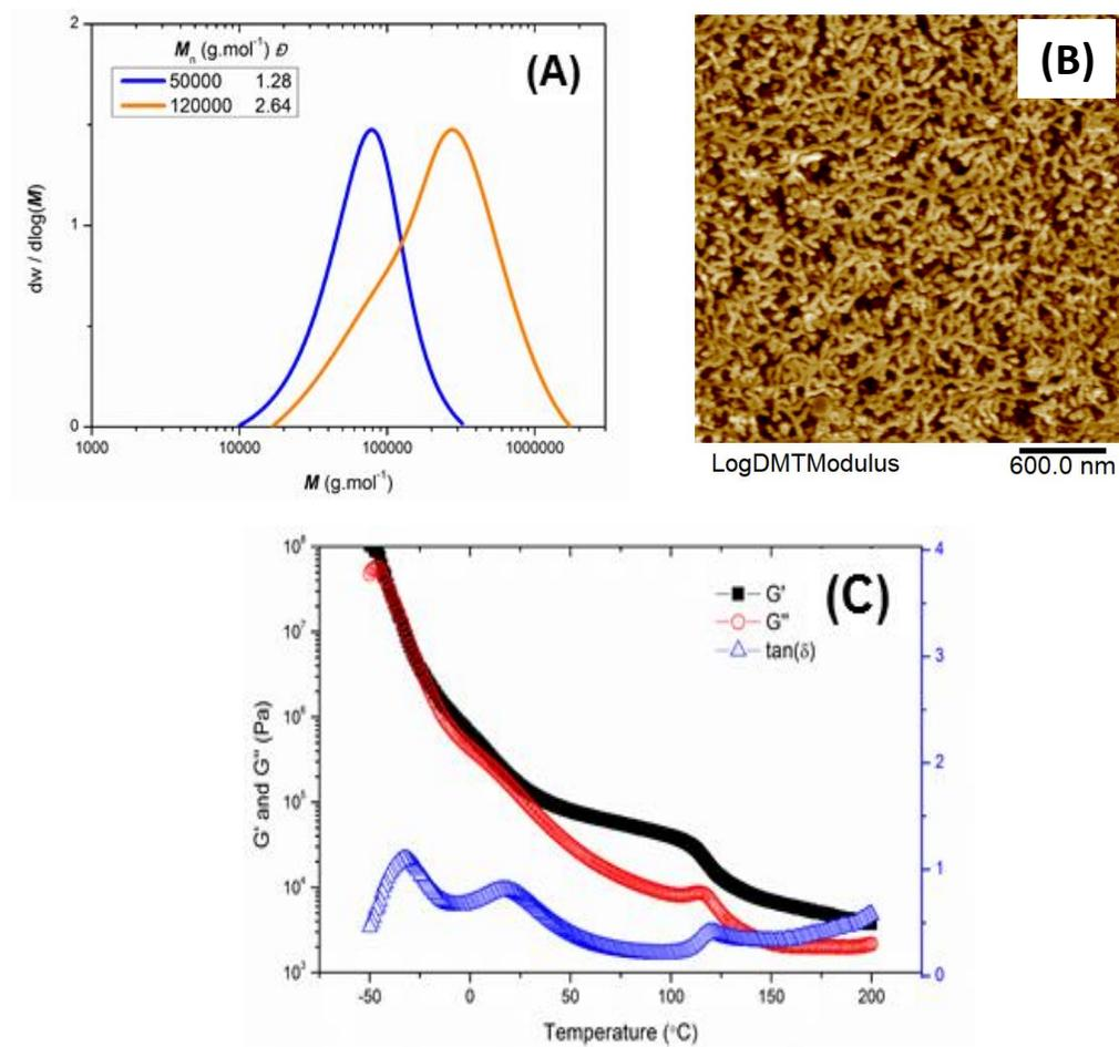
**Figure 4.5.** (A) SEC-MALS of PTHGA-*b*-PS-*b*-PTHGA. (B) AFM (PeakForce QNM mode) of PTHGA-*b*-PS-*b*-PTHGA. (C) Rheological behavior of PTHGA-*b*-PS-*b*-PTHGA with constant strain.
