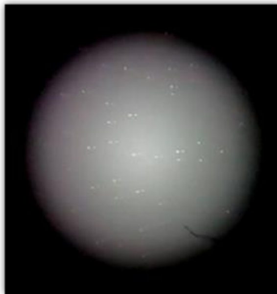
Figure A7. Stable droplet formation at Span 80 3% wt.
