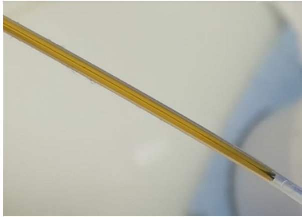
Figure B4. Clogging effect on the capillaries tips.
