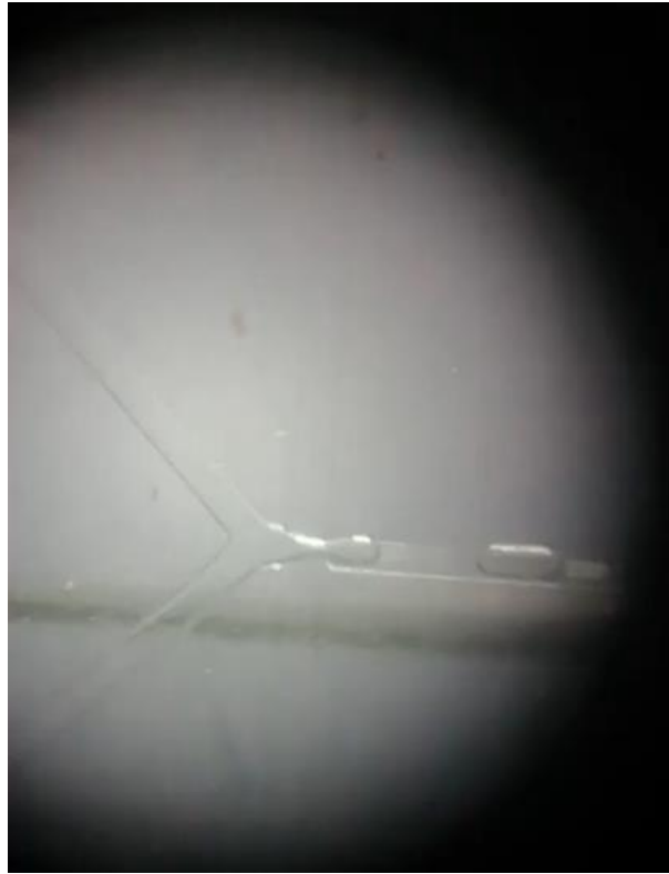
Figure A1. Squeezing regime forming aqueous slug formation.
