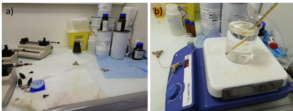
Figure 16. a) Microfluidic tubing reactor for Ag nanoparticles synthesis. b) Microfluidic tubing reactor for Au nanoparticle synthesis.
