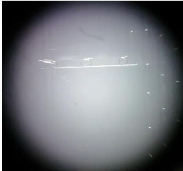
Figure A2. Dripping regime forming aqueous droplets.
