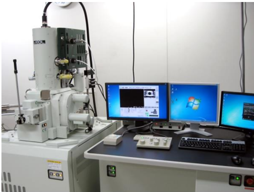
Fig. 2-10 Overview image of SEM, JSM-7100F (2-3).
