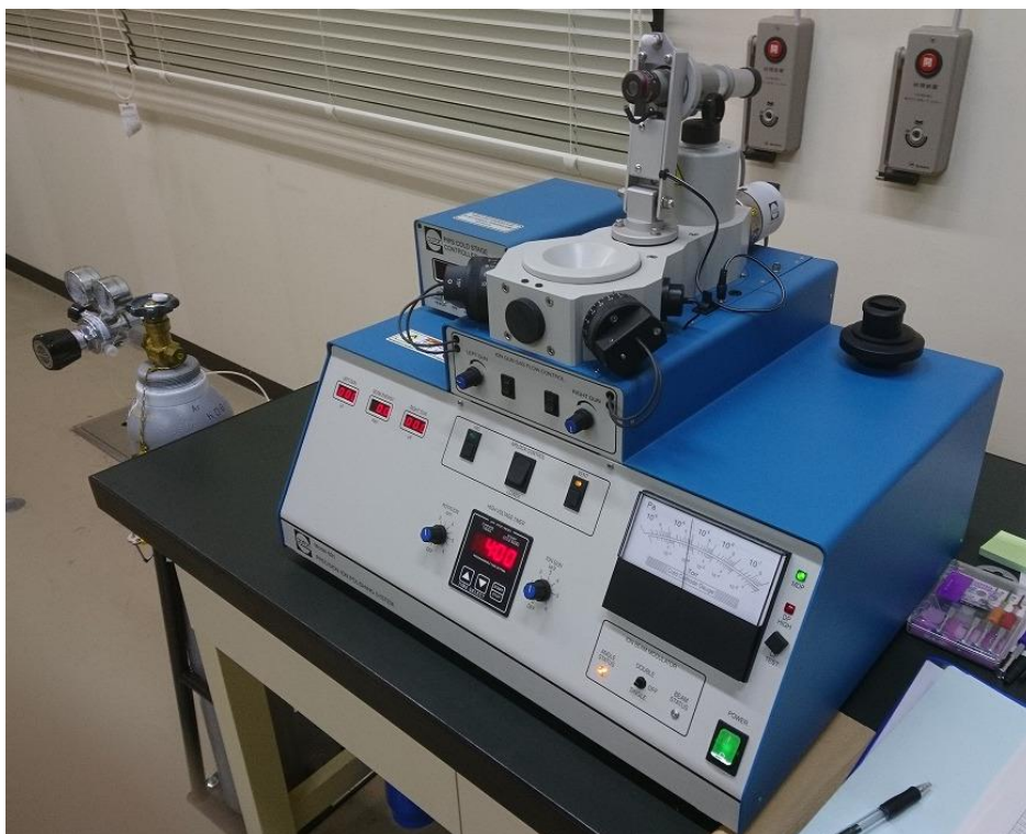
Fig. 2-7 Overview image of ion milling apparatus, PIPS Model 691
