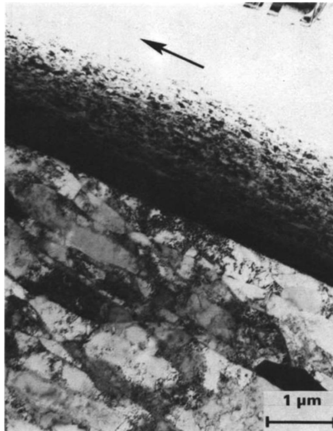
Fig. 1-10 TEM image of the cross-section of wear track showing ultrafine-grained mechanically mixed layer and elongated subgrains (1-22) .
