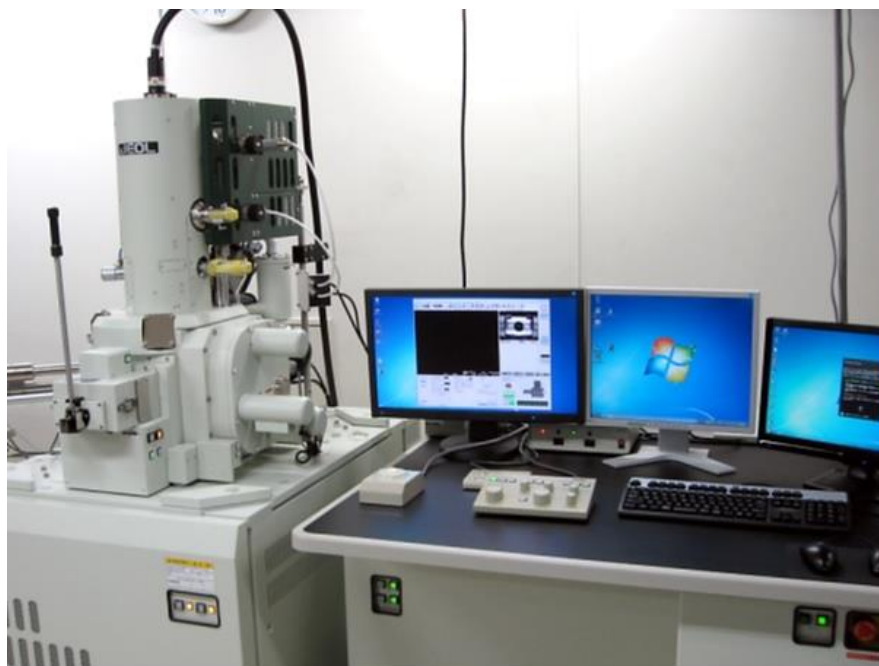
Fig. 2-10 Overview image of SEM, JSM-7100F (2-3) .
