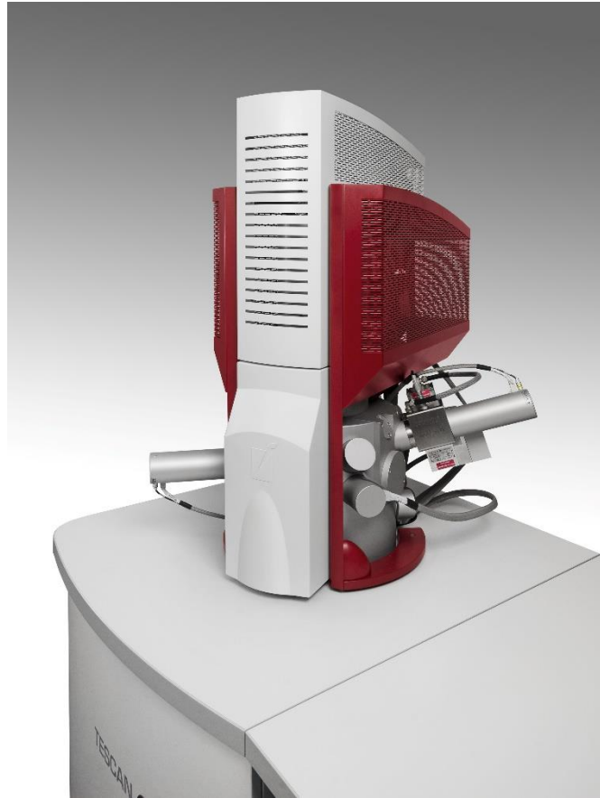
Fig. 2-11 Overview image of SEM, MIRA3 (2-4) .
