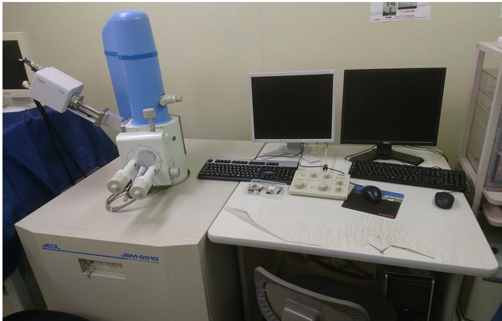
Fig. 2-9 Overview image of SEM, JSM-6510.
