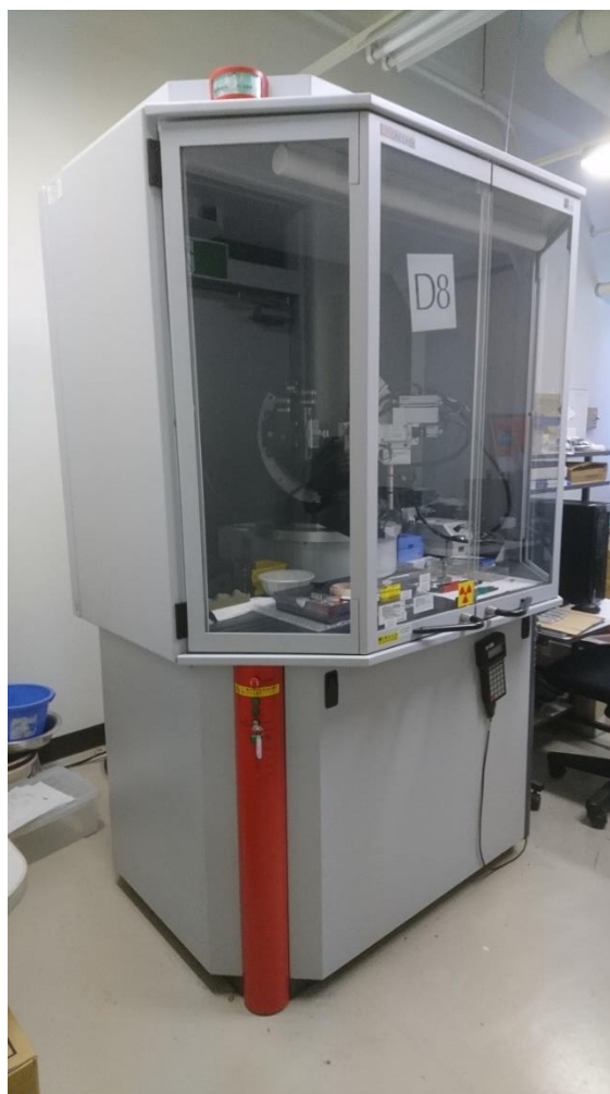
Fig. 2-16 Overview image of X-ray diffractometer (D8 Discover).
