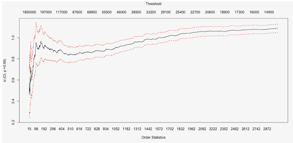
FIGURE 4.6 – Hill plot for the variable L . On the top, value of the threshold; on the bottom, corresponding rank of the observation in the sample.
