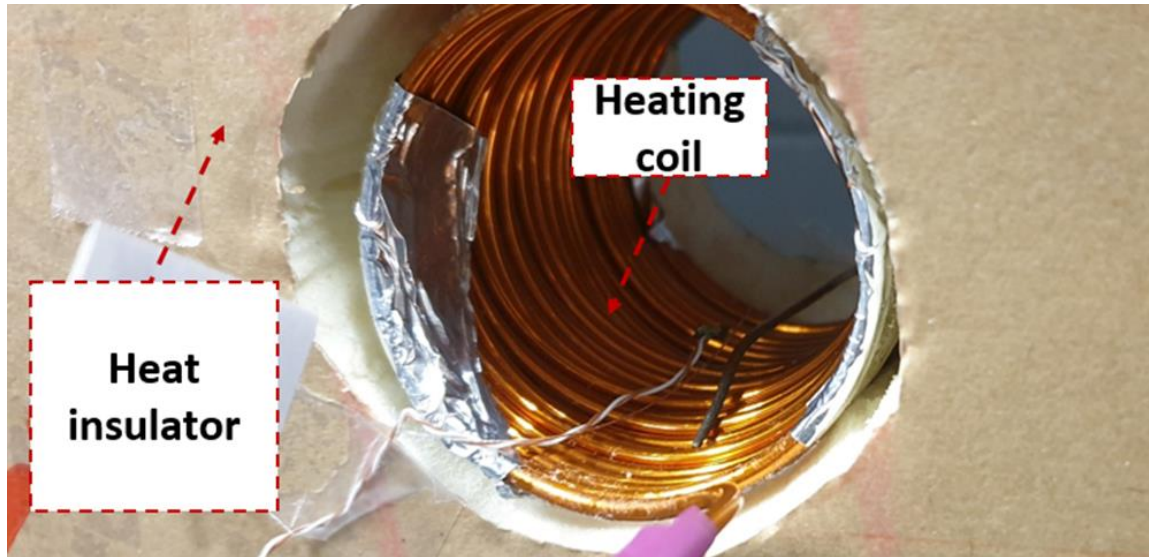
Figure 60: Heating system used for the FBG calibration
