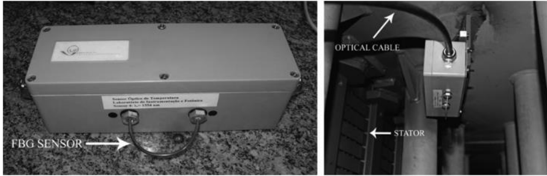
Figure 26: Box containing the optical fiber with the FBG inside the U-shape copper tubing (left) and installed inside the generator (right)
