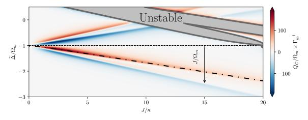
Figure 3.7: Predicted net permanent heat current  $Q_C$  in units of  $\Omega_m \times \Gamma_m$  around a ring of cavity-coupled optomechanical resonators as a function of the intercavity coupling and the detuning. The system is unstable in the grey region. The maximum current is found through the dash-dotted line. The lowest anti-Stokes sideband lies below, and is here identified by the arrow.
