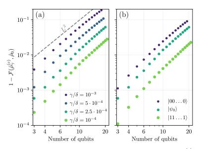
Figure 5.4: (a) Infidelity between the noisy output density matrix  $\rho_{\gamma}^{(c)}$  and the noiseless output  $\hat{\rho}_0 = |\text{GHZ}\rangle\langle\text{GHZ}|$  obtained from the initial state  $|\psi_0\rangle$  for different values of  $\gamma/\delta$ . The dashed line is a guide to the eye showing a growth  $\propto L^2$ . (b) Infidelity for three different initial states, described in the legend, for the same dissipation rate  $\gamma/\delta = 2.5 \times 10^{-4}$ .
