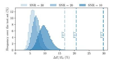
Figure 6.6: Frequency of the error score over the testing set for three SNR values averaged over 5 realisations of a  $20 \times 20$  photonic kernel machine.  $N_{\text{test}} = 3000$  for each realisation. The error score of the FFT is shown as dashed lines for comparison and falls systematically above the upper bound of that of the photonic kernel machine, in spite of being slower and requiring an ideal sampling rate significantly beyond the state of the art.
