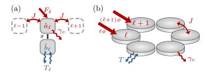
Figure 3.1: (a) Schematic representation of a single optomechanical cell and its nearestneighbour optical couplings.  $\hat{a}_{\ell}$  ( $\hat{b}_{\ell}$ ) is the optical (mechanical) mode of index  $\ell$ . (b) Ring of optomechanical disk resonators. Each site is optically driven with a phase that varies as  $\ell \phi$ , being  $\ell$  the site number. Optical modes are coupled while mechanical ones are not.
