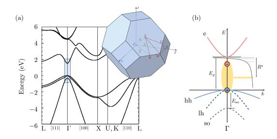
Figure 1.7: (a) Band structure of bulk GaAs, as computed in [147] with a 30-band  $\mathbf{k} \cdot \mathbf{p}$  method. (b) First Brillouin zone, as highlighted in (a), within a parabolic band approximation. The relevant conduction and heavy-hole bands are represented with plain lines. The first five electron-hole bound states are represented as dashed lines in the Coulomb potential. Adapted with permission from [148].
