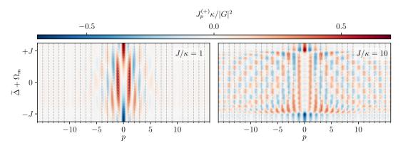
Figure 3.4: Dependence of the range of the cavity-mediated coherent interactions on the intercavity coupling and the detuning of the driving around the anti-Stokes sidebands.  $J_p^{(+)}$ , as given by Eq. (3.12), is shown for  $J/\kappa = 1$  (left pannel) and  $J/\kappa = 10$  (right pannel). The range of the interaction is found to be of the order of  $J/\kappa$ . Here L = 32, the rest of parameters are given in the text.
