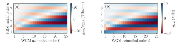
Figure 1.9: Electromechanical coupling in units of  $x_n^{\text{ZPF}}$  (panel (a)) and frequency units (panel (b)) for a disk of radius  $R_d = 1 \,\mu\text{m}$  and thickness  $L_z = 320 \,\text{nm}$  bearing a mechanical radial breathing mode of order n and an excitonic whispering gallery mode of order  $(p, \ell) = (1, \ell)$ .
