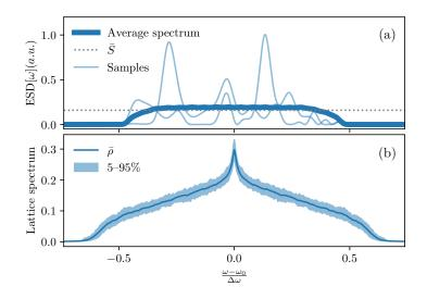
Figure 6.4: (a) Energy spectral density averaged over  $10^5$  realisations of the noiseless pulses, as given by Eq. (6.34), as well as that of a few individual realisations. (b) Mean and interval between quantiles 5% and 95% for the optical spectra of 100 realisations of a  $30 \times 30$  random photonic lattice.
