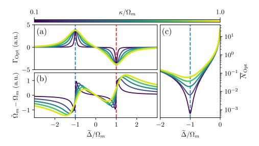
Figure 1.6: (a) Optical damping rate  $\Gamma_{\text{Opt}}$  as a function of the nonlinearly shifted detuning. Negative values correspond to positive gain. Cooling is maximal at the anti-Stokes sideband (dashed blue line); conversely, heating is maximal at the Stokes sideband (dashed red line). (b) Optical spring effect (Lamb shift) as a function of the nonlinearly shifted detuning. (c) Effective Planck thermal population associated to the optical "thermal bath" around the anti-Stokes sideband.
