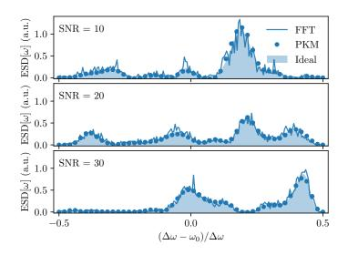
Figure 6.7: Worst-case predictions of a  $20 \times 20$  photonic kernel machine (dots) over the testing set. The ideal noiseless energy spectral densities to be reconstructed (shaded area) and those obtained by squaring the FFT of the noisy input pulse (plain line) are shown for comparison. Normal-mode populations are measured.  $N_{\text{test}} = 3000$ .
