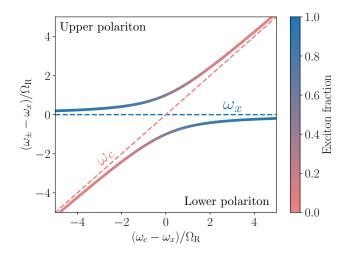
Figure 1.10: Upper and lower polariton angular frequencies as a functions of the frequency mismatch between the cavity photons and the quantum-well excitons. At  $\omega_c \approx \omega_x$ , the spectrum exhibits an avoided crossing due to the optoelectronic interaction that separates the two branches by twice the Rabi splitting  $\Omega_{\rm R}$ .
