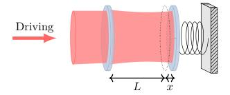
Figure 1.4: Schematic representation of a Fabry-Pérot-based cavity optomechanical system. Photons circulate between the harmonically confined mobile end mirror and the input mirror through which photons are pumped into the cavity.
