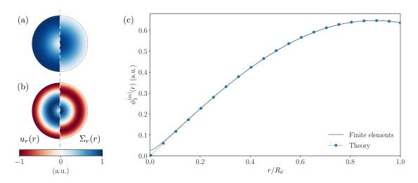
Figure 1.2: Radial displacement  $u_r(r)$  and strain  $\Sigma_r(r) = \nabla_r \cdot \boldsymbol{u}(r)$  associated to the (a) n = 1 and (b) n = 2 radial breathing modes. (c) Comparison of the theoretically derived phonon wave function and that obtained by finite-element calculations for a GaAs disk of radius  $R_d = 2 \,\mu\text{m}$  and thickness  $L_z = 300 \,\text{nm}$ .
