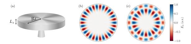
Figure 1.1: (a) Semiconducting optomechanical nanodisk resonator on its pedestal. In-plane view of its optical whispering-gallery modes, as given by Eq. (1.6), for (b)  $p = 1, \ell = 15$ , and (c)  $p = 2, \ell = 10$ .
