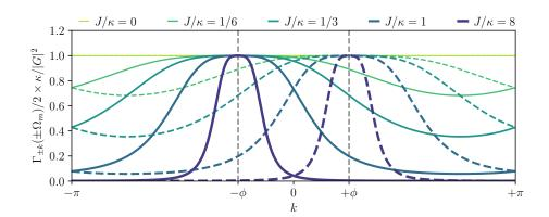
Figure 3.5: Gain  $\Gamma_{-k}(-\Omega_m)$  (dashed) and loss  $\Gamma_k(+\Omega_m)$  rates induced by the engineered reservoir for various  $J/\kappa$ .  $\tilde{\Delta} = +\Omega_m - J$  for the gain rate and  $\tilde{\Delta} = -\Omega_m - J$  for the loss rate. Here L = 8, the rest of parameters are given in the text.
