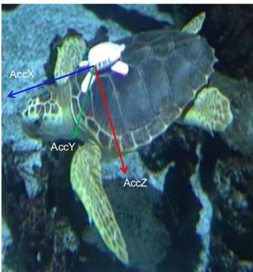
Fig. 1. Accelerometer attachment. A captive loggerhead turtle equipped with a bio-logger (WACU) attached to the carapace using waterproof double-backed adhesive tape. The three arrows indicate the axes measured by the accelerometers.
