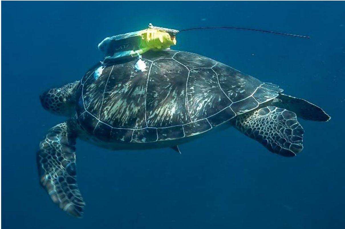
Supp. Figure 1. Free-ranging immature green turtle equipped with a device combining a high-frequency tri-axial accelerometer, a high-frequency tri-axial gyroscope, a depth recorder and video-recorder.
