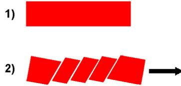
Figure 1.1: Slip mechanism illustration in plastic deformation.
