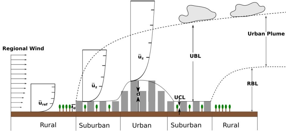
Figure 2.17: Schematic representation of two-layer urban atmosphere classification combined with the vertical wind profiles, adapted from: [90] and [93].
