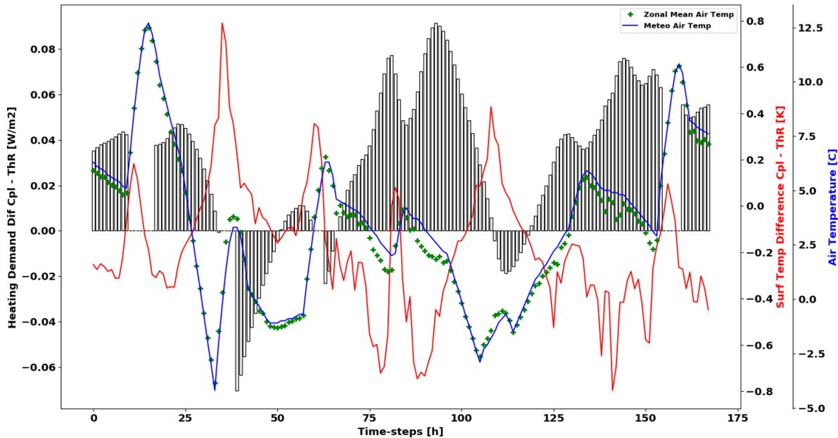
Figure 4.15: Heating demand difference as a function of surface temperature difference and air zonal temperature for a referenced zone during a representative heating week between CS1a\_NF and CS1a\_ThR scenarios.
