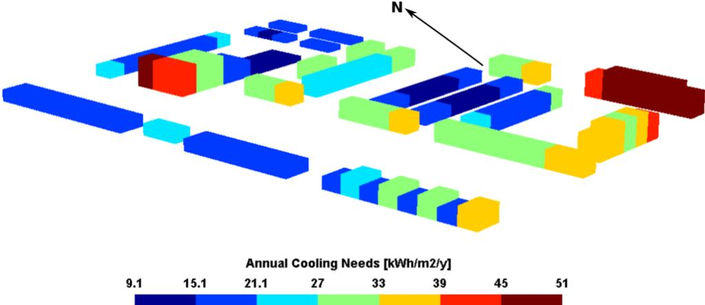
Figure 5.25: 3-D visualization of cooling needs per building for the DEN\_2050 scenario.
