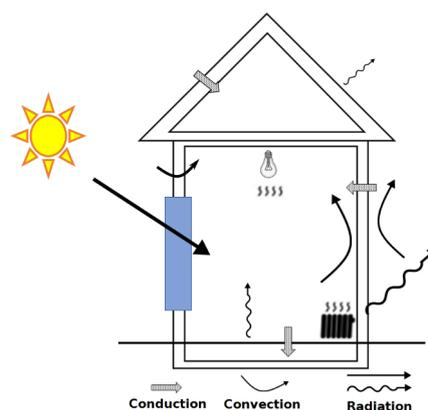
Figure 2.3: Heat transfer balance on a building.
