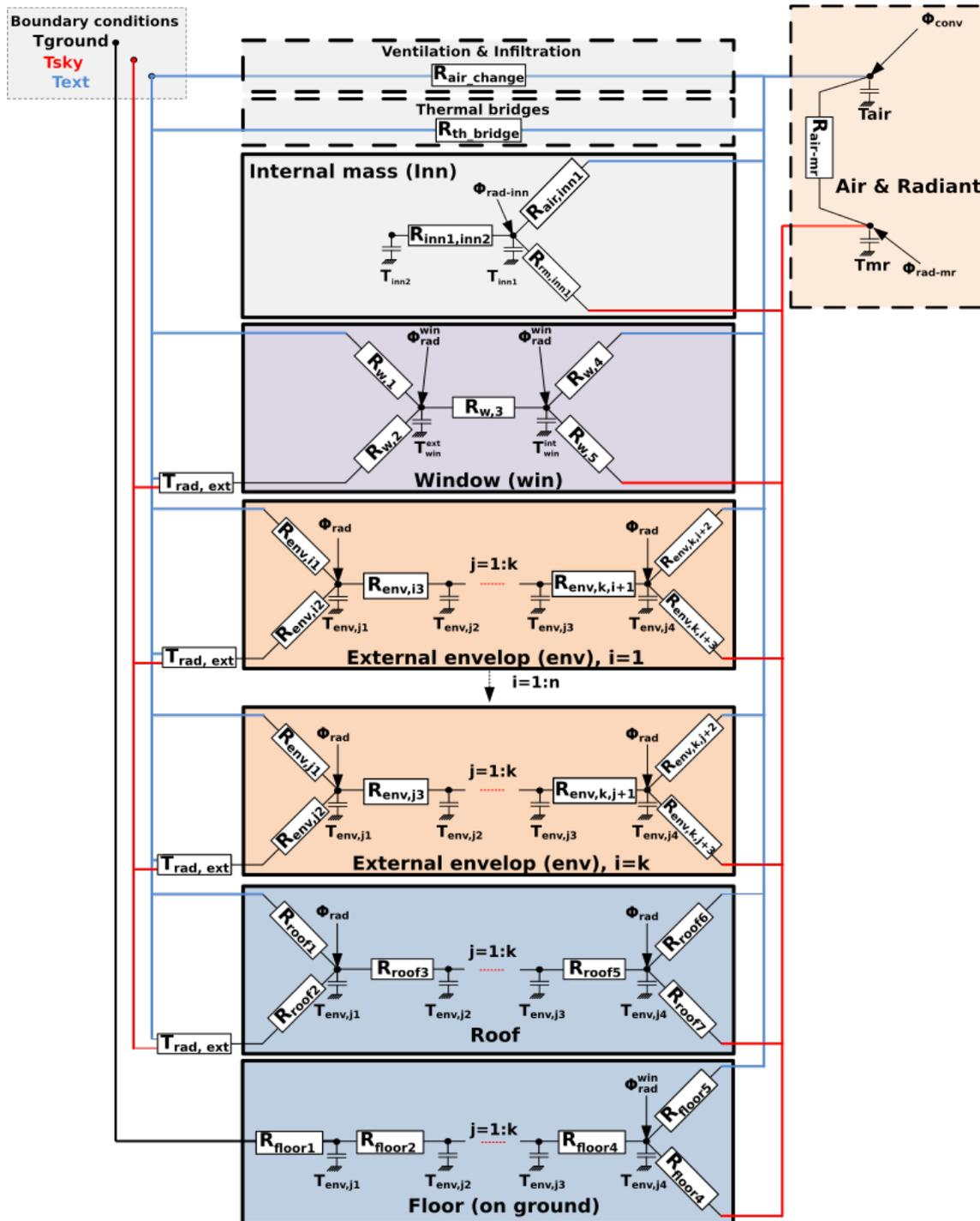
Figure 3.1: Layout of the thermal zone model, adapted from [182].
