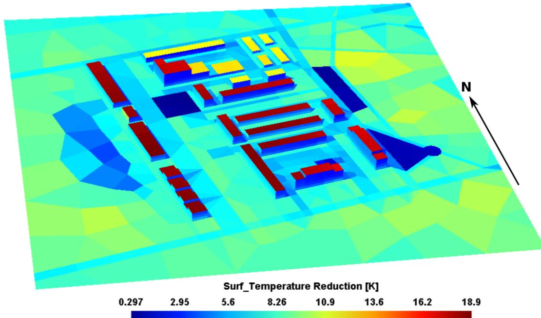
Figure 5.39: Visualization of the surface temperature difference between the conventional and the highly reflected urban surfaces during the maximum air temperature of the extreme scenario.
