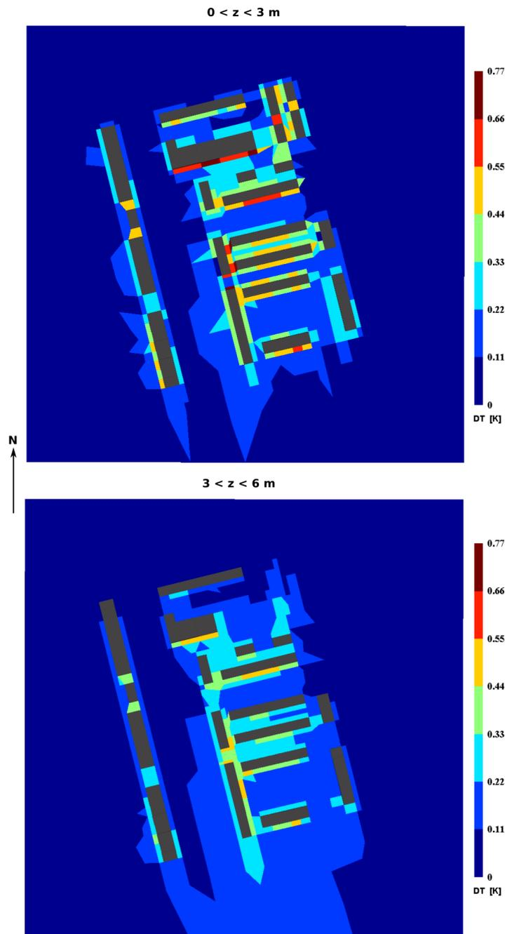
Figure 5.19: 3-D visualization of the air temperature difference [K] between the AC\_Std and the DEN\_Std simulation scenarios for two horizontal canopy layers during the hottest time step of the meteorological file.
