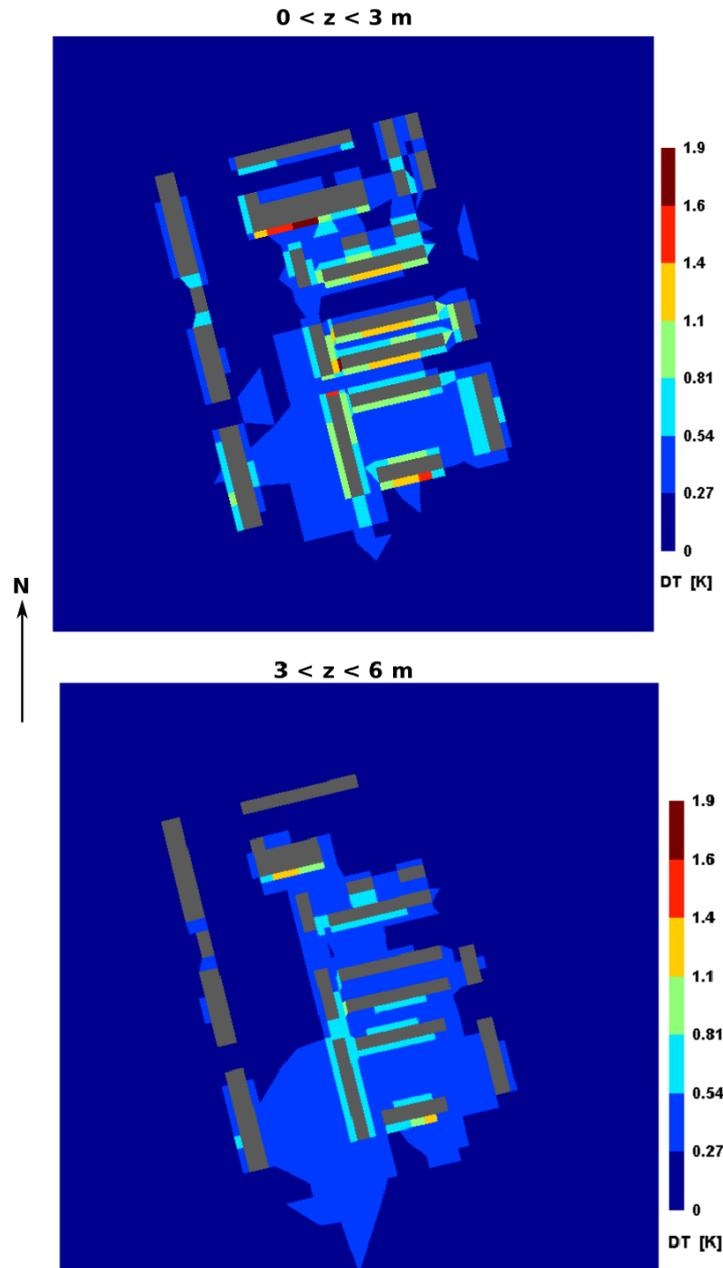
Figure 5.28: 3-D visualization of the air temperature difference [K] distribution between the AC\_2050 and the DEN\_2050 simulation scenarios for two horizontal canopy layers during the hottest time step of the meteorological file.
