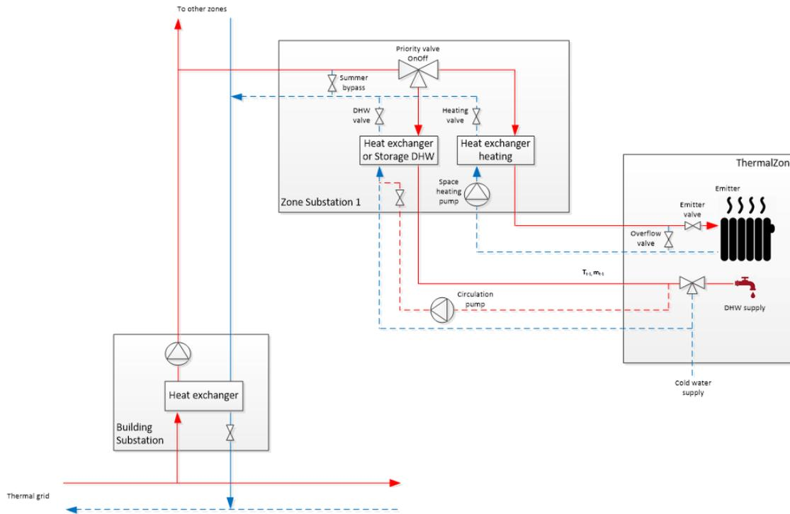
Figure 3.5: Schematic representation of a centralized energy generation scheme with building & zone substations, source: CSTB.
