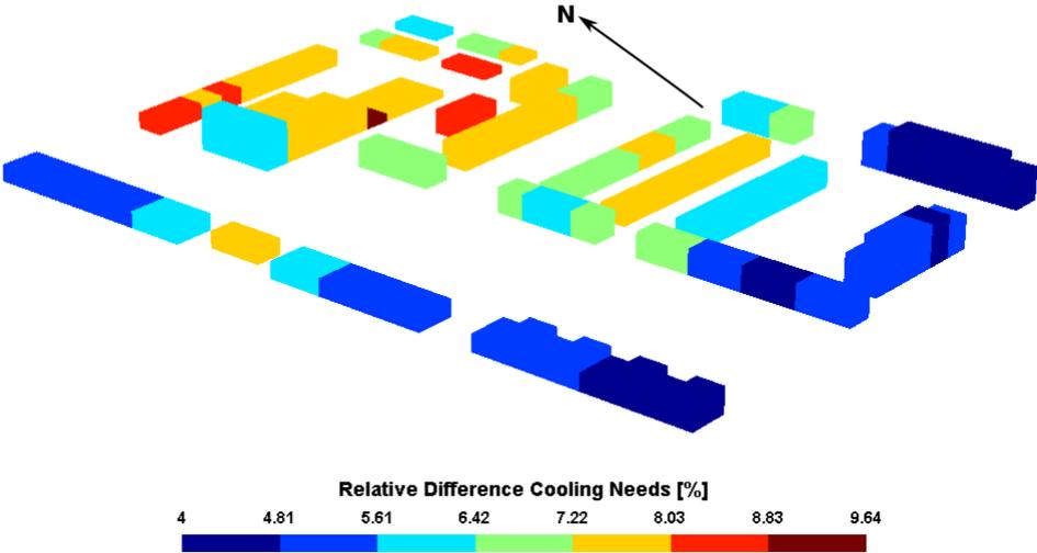
Figure 5.26: 3-D visualization of the relative difference on cooling needs per building for the implemented extreme scenarios.
