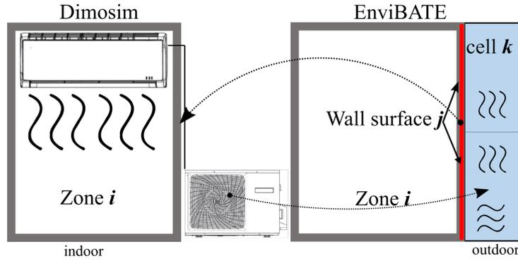
Figure 4.3: Schematic representation of the exchanged variables.
