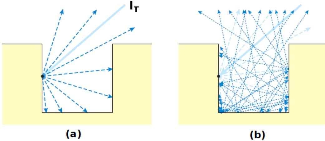
Figure 2.12: Schematic representation of (a) first reflection and (b) second reflection of beam component from a canyon facets, source: [65].
