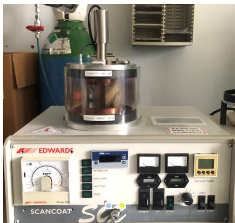
Figure 29: Sputtering machine used for metallization
