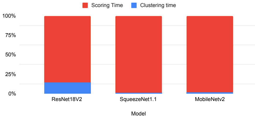
Figure 4.5: Profiling simulation time between the k -means clustering application and the scoring of approximate candidates using the validation dataset for Algorithm 1.
