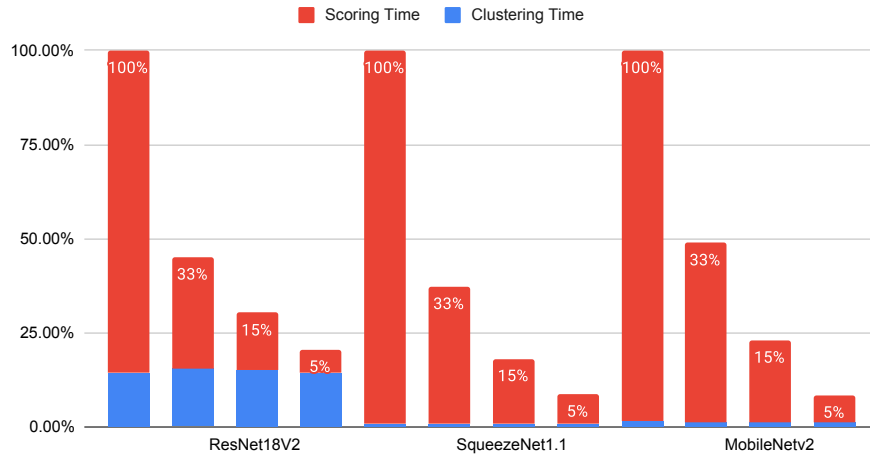
Figure 4.7: Profiling simulation time between the k -means clustering application and the scoring of approximate candidates using the validation dataset for Algorithm 2.
