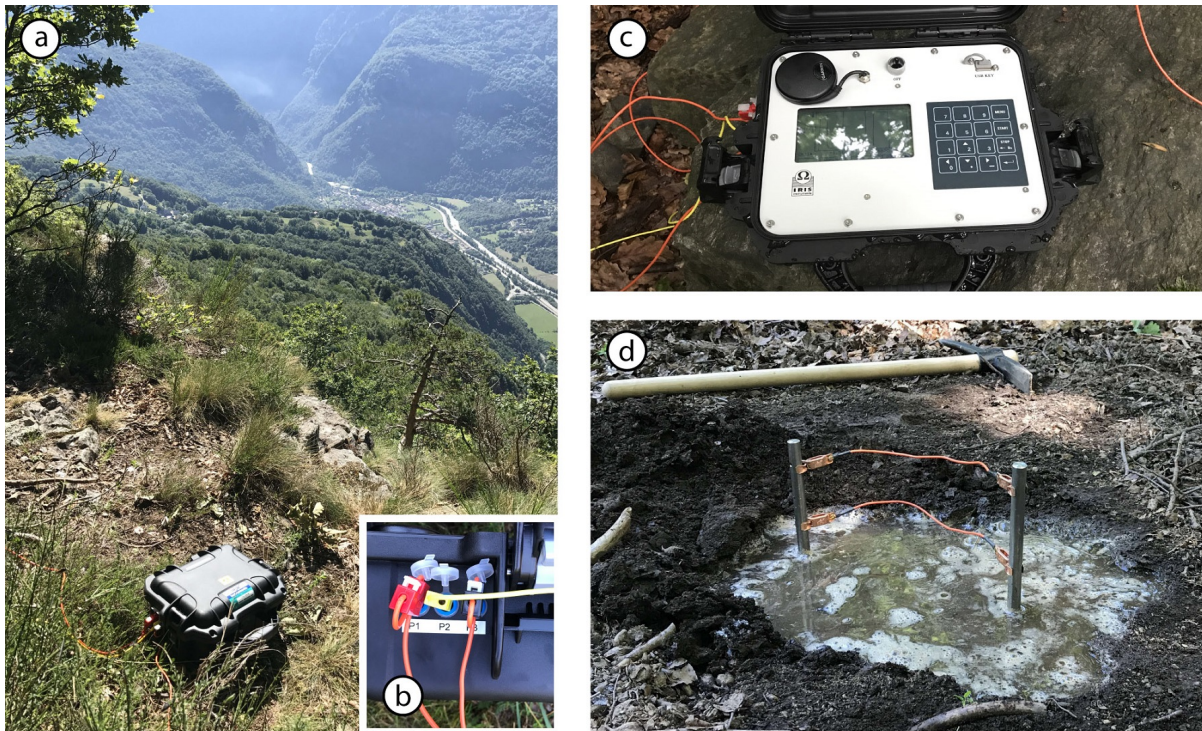
Figure 4.2: Photographs of the monitoring equipment and of the measurement sites: (a) V-FullWaver unit at position FW9; (b) Zoom on the plugs for the three measurement channels on a V-FullWaver unit; (c) Zoom on the control screen of a V-FullWaver unit; (d) Remote electrode fully watered with a highly conductive salted mixture.
