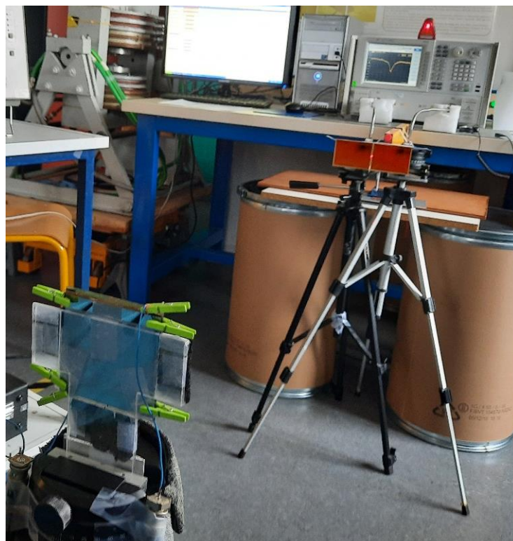
Figure 4.2.5 Illustration of the method that was used to adjust the orientation of the DUT by using laser pointer between and just behind the two horns (normal direction with respect to the DUT) with monitoring of the reflected laser spot
