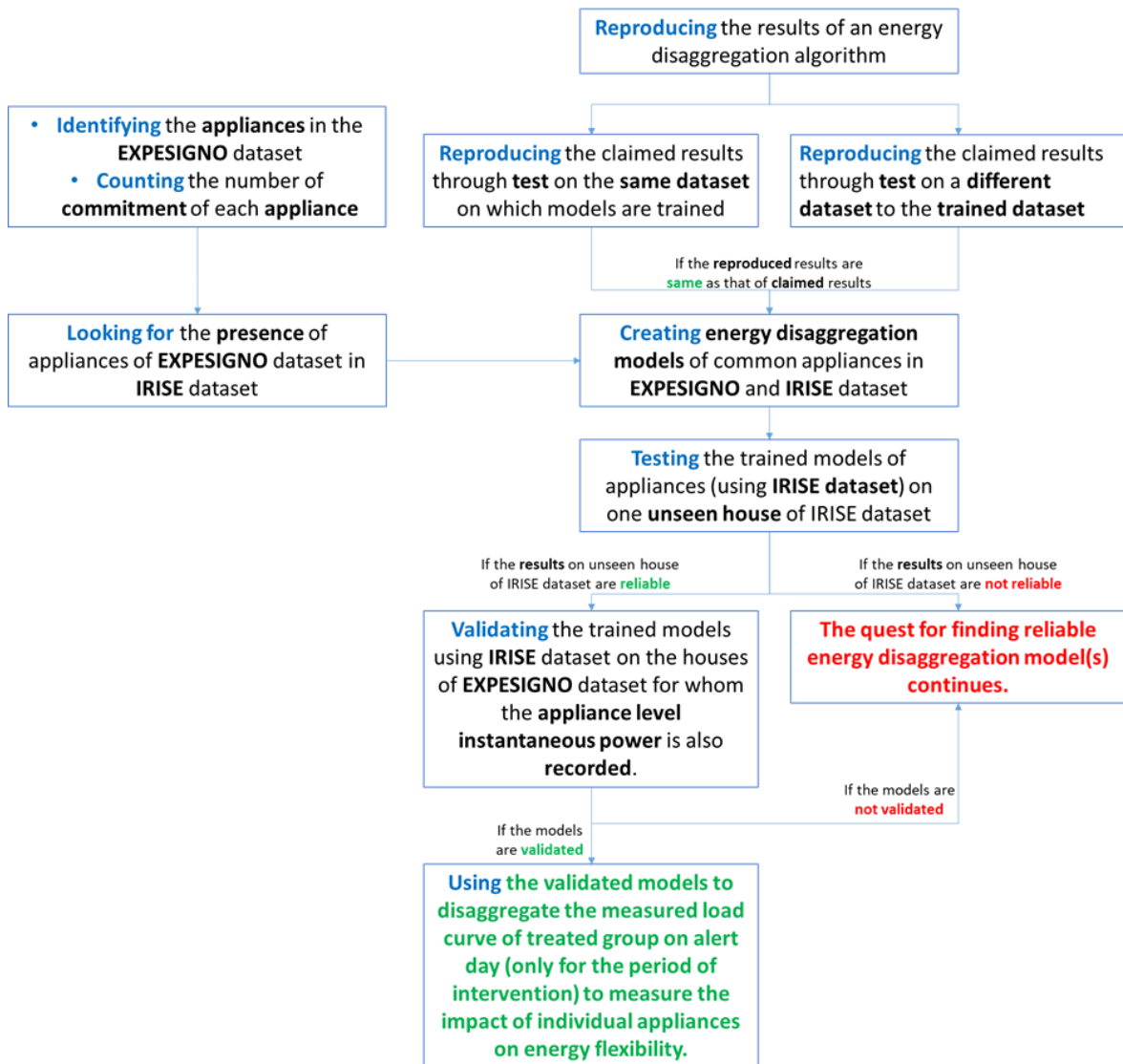
Figure V.2 Schematic diagram of energy disaggregation of measured load curves on alert days
