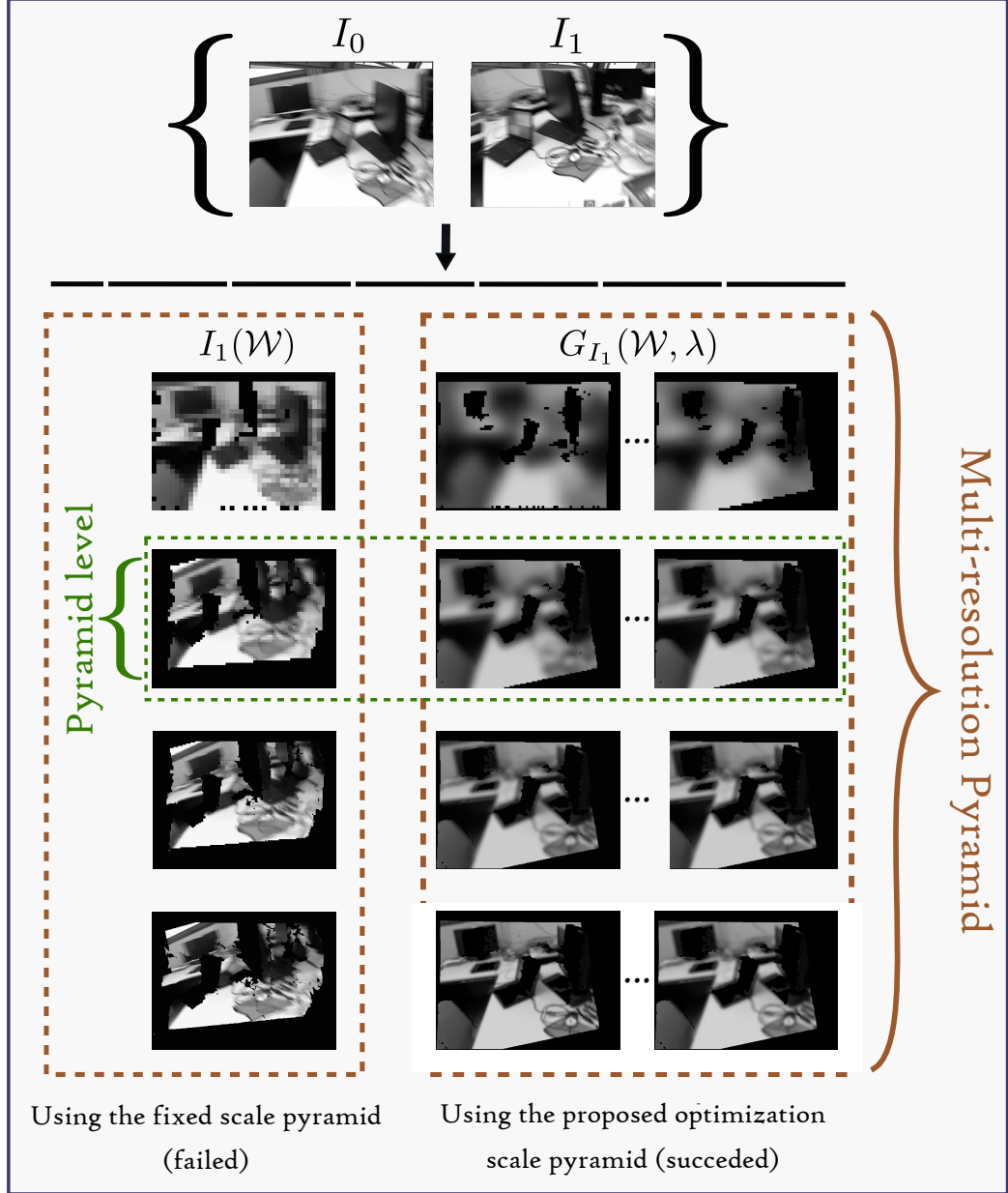
FIGURE 6.1: The considered algorithms aim at aligning the image pair \{I_0, I_1\} , where the images resulting from the alignment are G_{I_1}(\mathcal{W}, \lambda) and I_1(\mathcal{W}) . Here the fixed scale pyramid-based method (PP-B) was unable to align the image pair because it fell in a local minimum, while the proposed optimized scale pyramid-based method (OP-B) succeeded because it is able to automatically adapt the image smoothing to suppress local minima.
