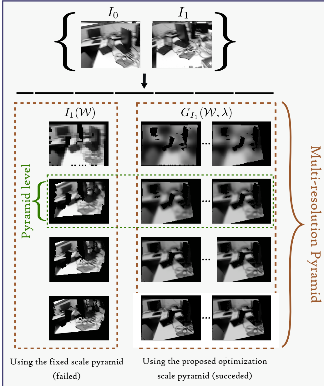
FIGURE 6.1: The considered algorithms aim at aligning the image pair \{I_0, I_1\} , where the images resulting from the alignment are G_{I_1}(\mathcal{W}, \lambda) and I_1(\mathcal{W}) . Here the fixed scale pyramid-based method (PP-B) was unable to align the image pair because it fell in a local minimum, while the proposed optimized scale pyramid-based method (OP-B) succeeded because it is able to automatically adapt the image smoothing to suppress local minima.
