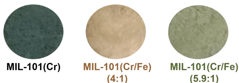
Figure 3-16: Photos of the powders of MIL-101(Cr), MIL-101(Cr/Fe) (4:1) and MIL-101(Cr/Fe) (5.9:1).
