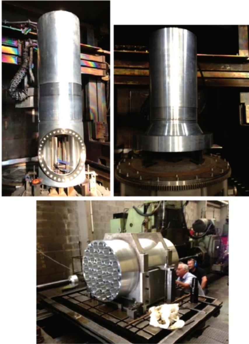
**Figure 1.2:** *Component of RJH reactor - part of core fabricated using 6061 T6 aluminum alloy.*
