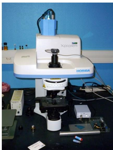
FIGURE A2: Microscope Raman confocal (Horiba Jobin-Yvon), modèle XploRA.
