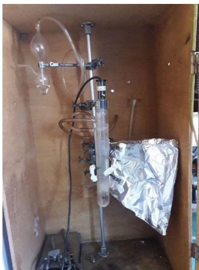
Figure II-16: lampe « Hanau TG 150 High-pressure mercury arc lamp »
