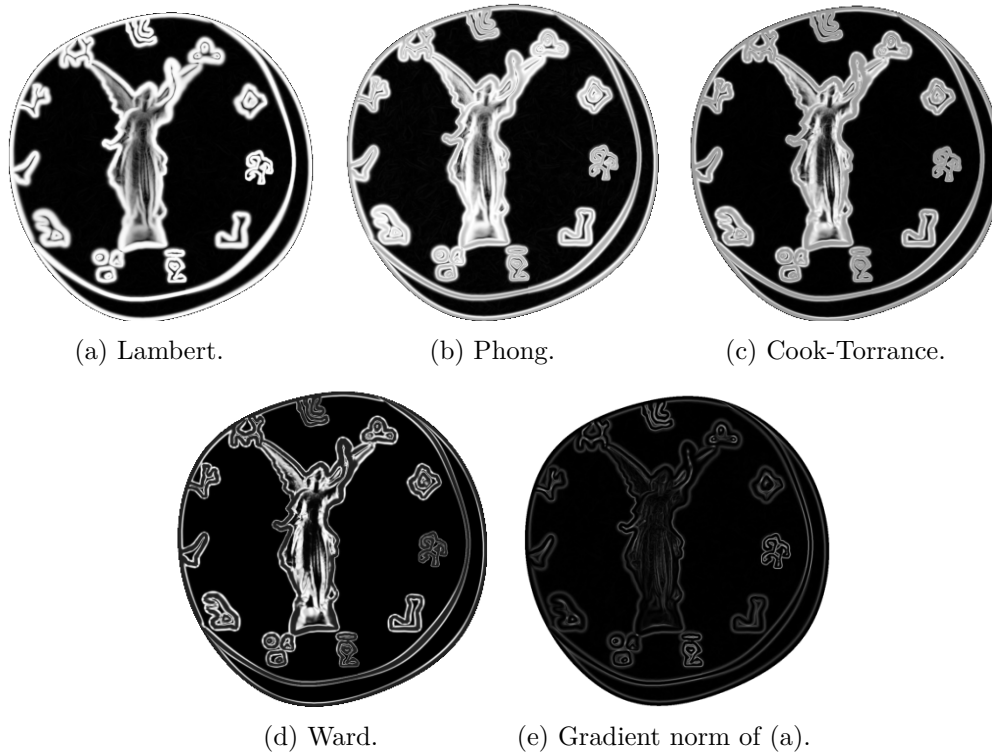
Figure 2.32: Energy maps for four types of BRDFs with increasing specularity and gradient magnitude of the Lambertian energy map.
