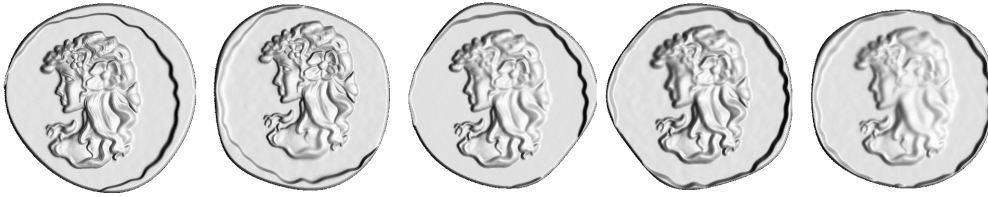
Figure 2.23: Five examples of coins from the same die, in order of creation. One die is used to make 5 coins and wears out in the process, leading to less detailed versions of the coin.
