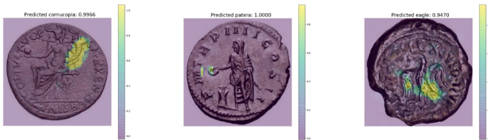
Figure 1.8: Salient regions learned with the neural network structure proposed by Cooper et al. [27] (Figure 8). According to the authors, the learning is adequately correlated with visual symbolic content within the coins which would enable a relevant, symbol-based recognition.
