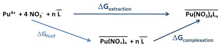
FIGURE 12 – Cycle thermodynamique : extraction vs complexation
