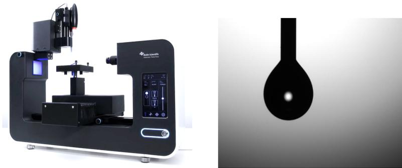
**Figure 2.6:** Left: Tensiometer used to measure precise surface tension of used liquid. Right: droplet released from Gauge needle in front of high resolution camera to measure instantaneous surface tension .
