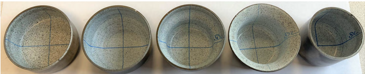
Figure 3.9 – Different steps of measurement for the redrawing process (from left to right: end of the stage 1, stage 2 with a punch stroke of respectively 5, 15 and 25 mm, end of the stage 2)
