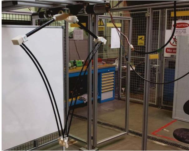
FIGURE 1.4 – Robot parallèle souple, [CAMPA et al., 2019].
