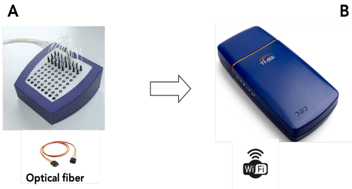
Figure 2.15: Optimization of HD-sEMG acquisition chain from REFA amplifier (A) to Mobita ambulatory device (B).
