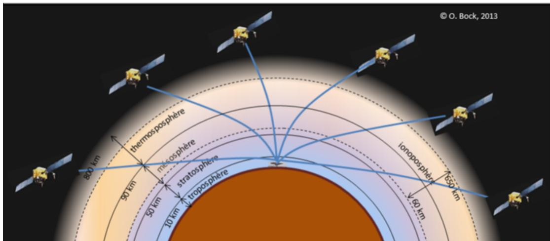
Figure B.1 – Propagation of GPS signals. Source Bock, 2013.
