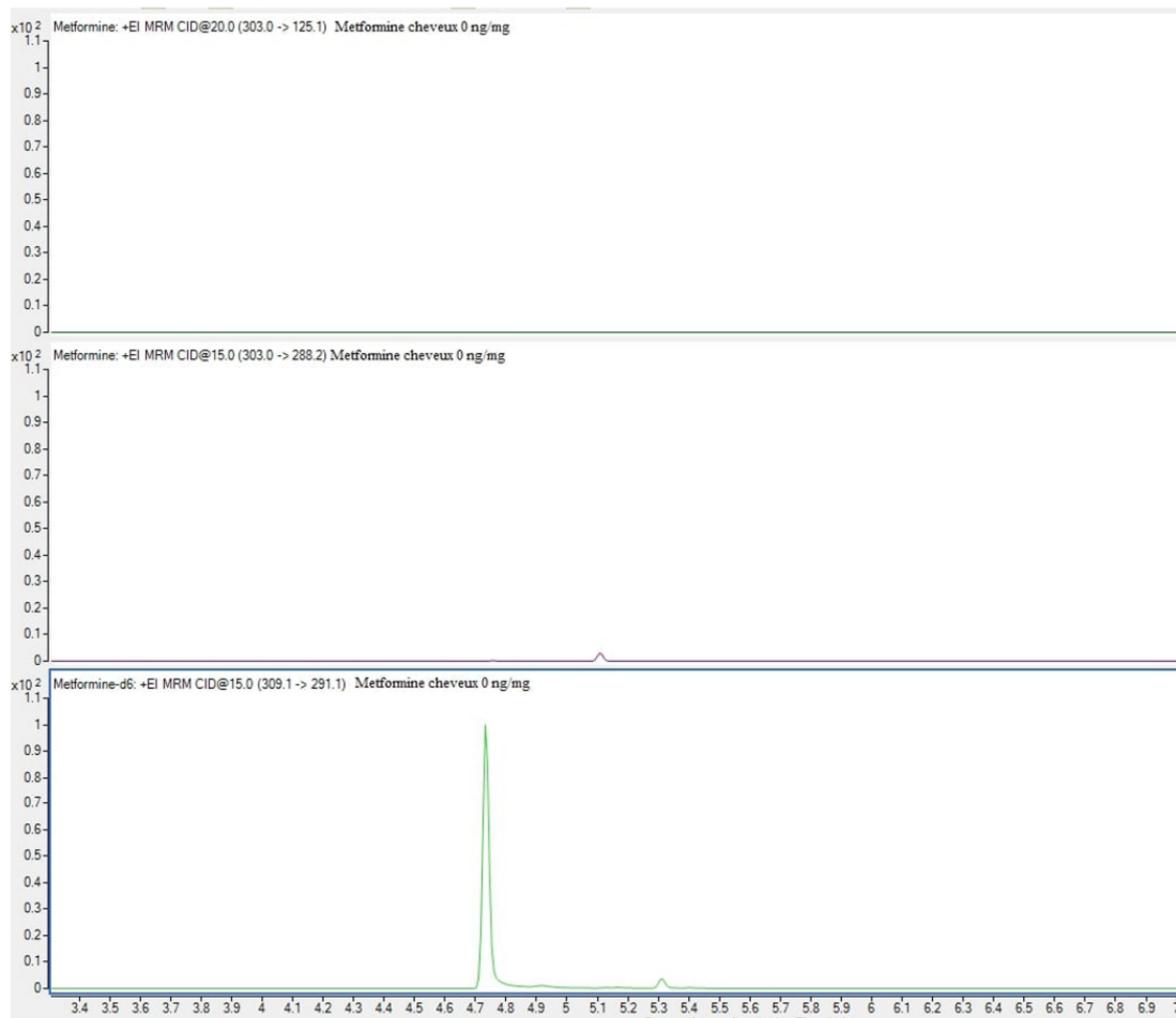
FIGURE 2 Chromatogram of blank hair sample (from top to the bottom: 2 transitions of metformin and 1 transitions for IS metformin-d6) [Colour figure can be viewed at wileyonlinelibrary.com ]
