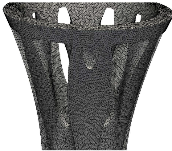
Figure 7.12: Mesh of the shape (7.10b)
