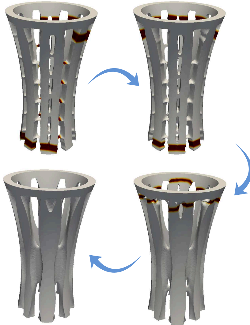
Figure 1.6: Intermediate shapes encountered while finding a crack-free optimal column (black zones represent cracks)
